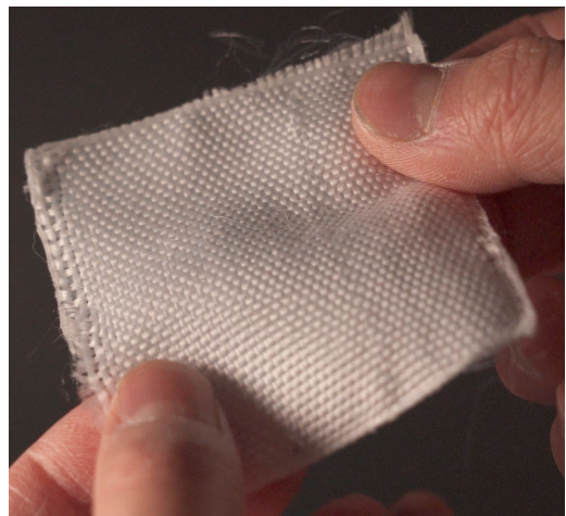
Figure 12: (Top, bottom left) Weaving PE fabric on an Ashford 16" rigid heddle loom; (Bottom right) Sample swatch of plainweave PE fabric.
