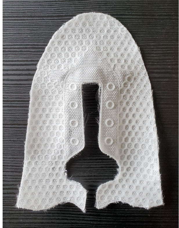
Figure 16: (Left) Sample 3D printable sneaker upper pattern with variegated hexagonal pattern,;(Right) fabricated mono-PE 3D-PPOT sneaker upper pattern.
