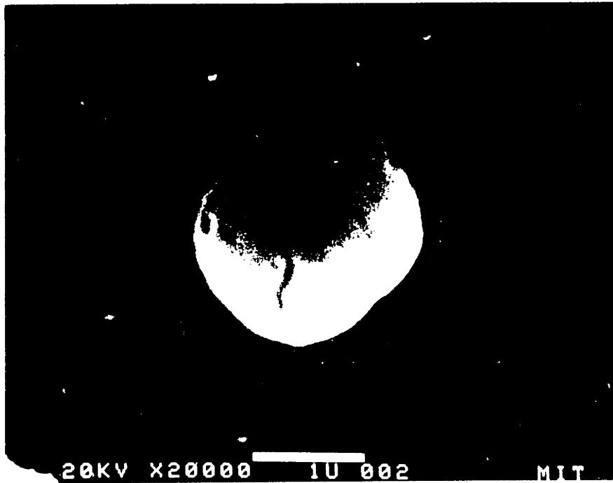
Figure 8.2: SEM Micrograph of Witness Strip Coated Alongside Moisture Sensor Z3 a) Scale 52 mm = 100 \mu m (500X), b) Scale 11 mm = 1 \mu m (20,000X).
