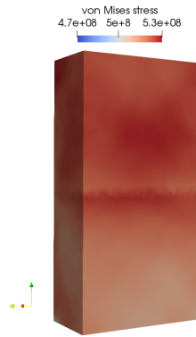
(a) von Mises stress at a bi-crystal cross section parallel to x - z plane at \epsilon = 0.3\%
