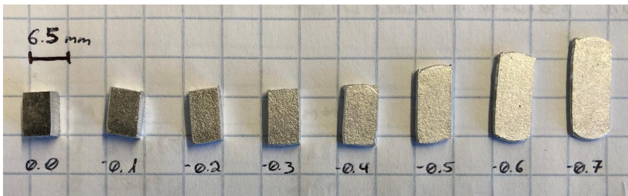
Figure 2-3: Annealed, rolled aluminum samples listed by approximate strain level
