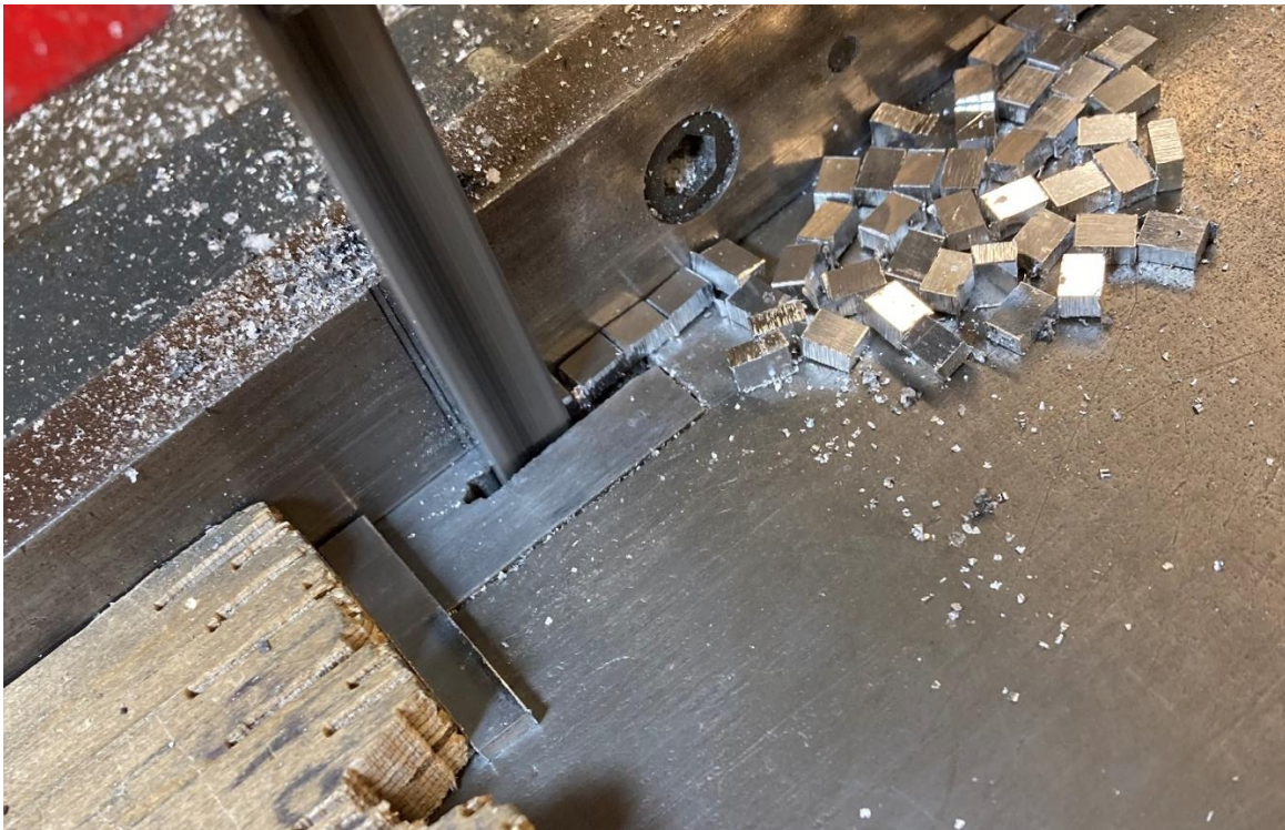
Figure 2-1: Samples pile up on the far side of a bandsaw's blade after being cut from the thin bar of aluminum just in front of the wood push block.
