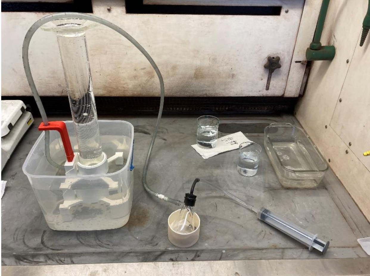
Figure 2-7: Image of the test setup used. In the back right are beakers of DI water for refilling the syringe and wetting the rubber stopper and a rectangular dish of tap water to cool the Buchner flask after the reaction.
