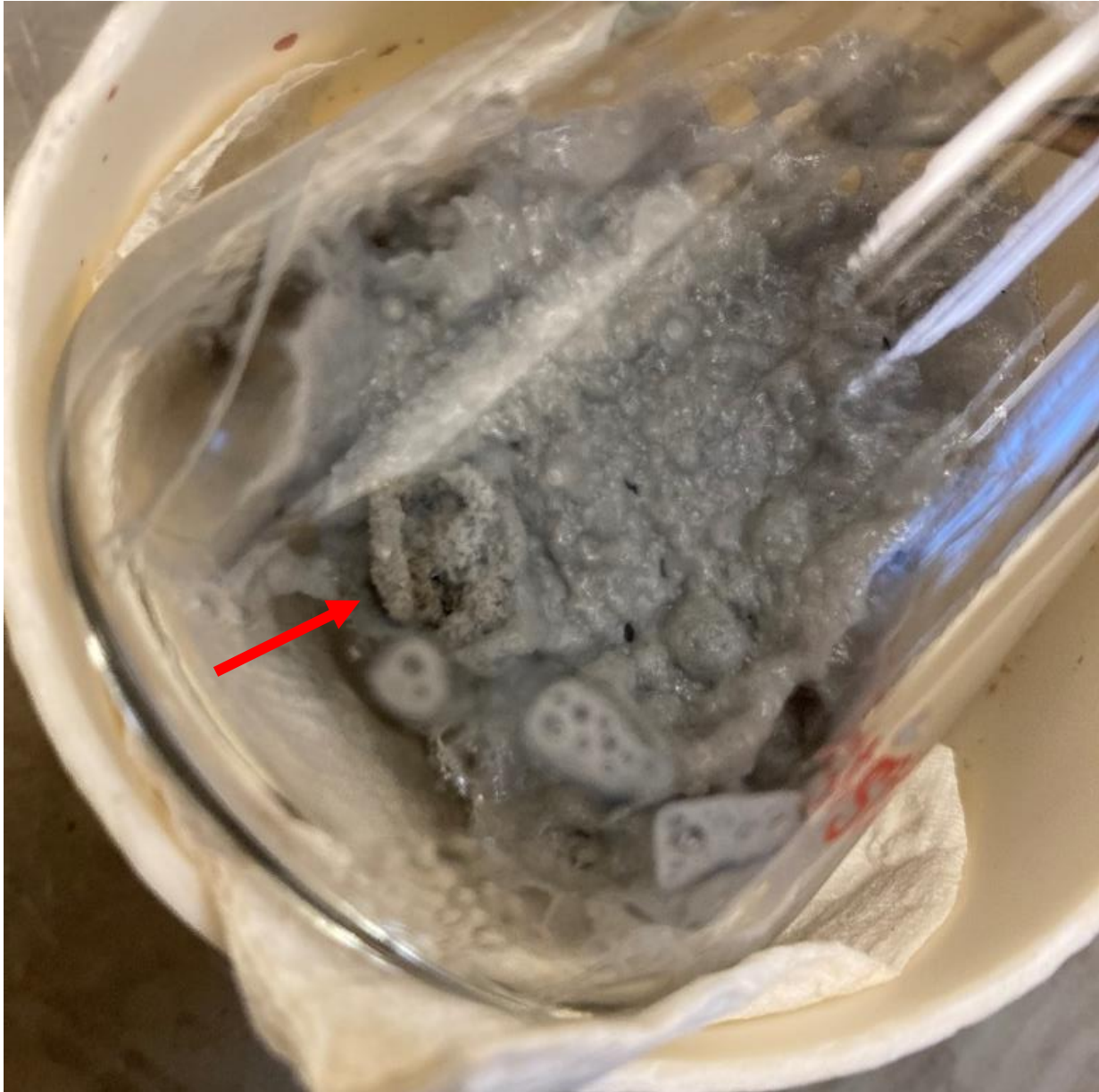
Figure 2-8: A sample of aluminum with a high strain level of 0.6, reacting in DI water, has been thrown to the top of the products and dried out, prematurely halting the reaction.
