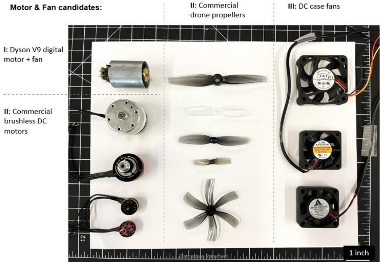
FIG. 18. Summary of motor and fan candidates for high-efficiency air delivery. Three groups of solutions were explored in parallel. (I): Dyson V9 digital integrated motor fan. (II): Commercial brushless DC motors combined with commercial drone propellers. (III): DC computer case fans.
