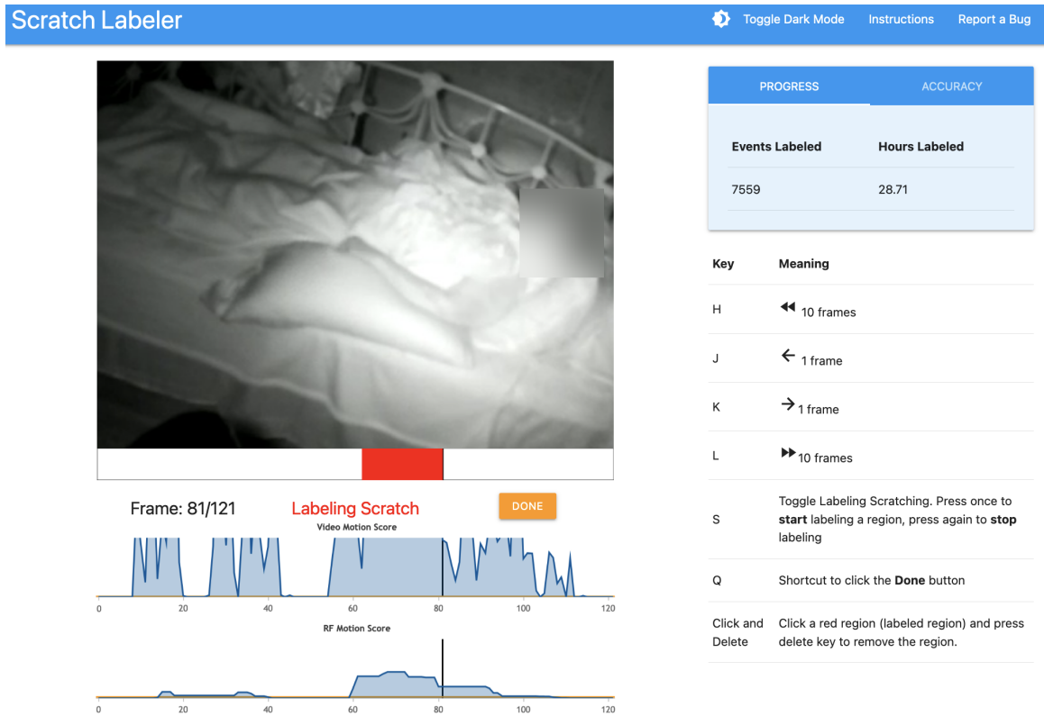
Figure 4-1: An example of the labeling server developed for annotating scratching events based on the collected infrared footage.
