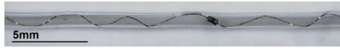
Figure 7-9: Photograph of a temperature sensing fiber with a thermistor connected to buckled electrodes.
