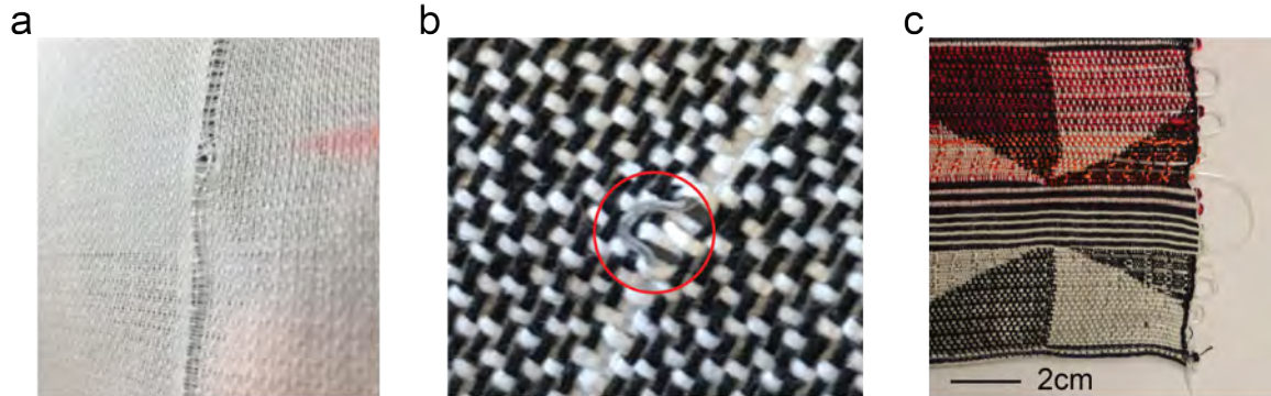
Figure 6-2: (a) Fabric deformation and (b) fiber buckling after weaving a PC fiber in a cotton fabric. (c) Loops of PC fibers at the end of a weave.
