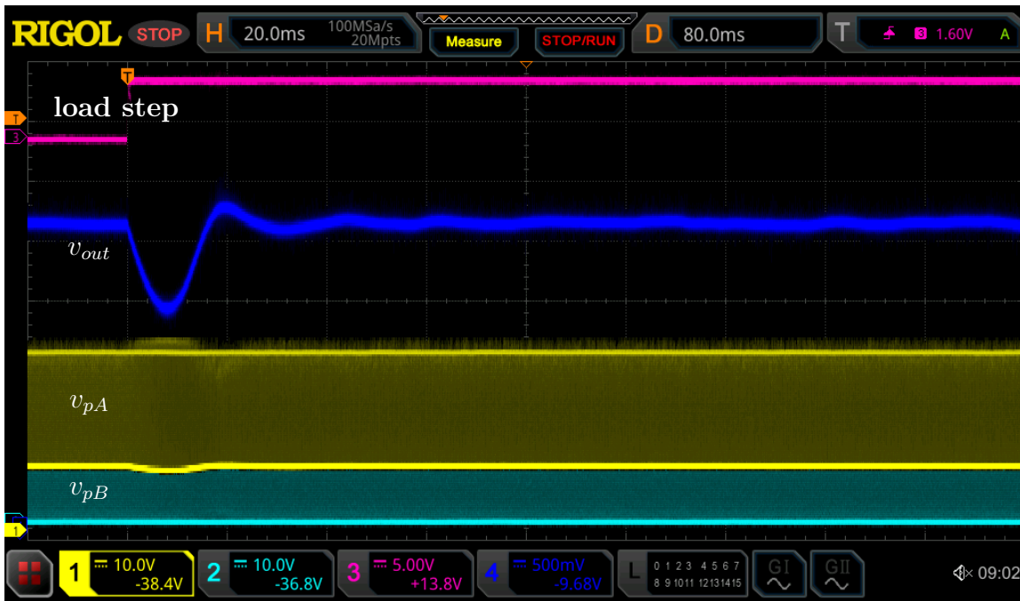
Figure 4-12: Experimental transient response to R_{load} step from 600\ \Omega to 300\ \Omega with V_{in} = 30\ \text{V} and V_{cmd} = 10.4\ \text{V} . The peak deviation from steady state is 770\ \text{mV} (7.5% of V_{cmd} ) and the 2% settling time is 14.6\ \text{ms} . Figure source: Joshua Piel.
