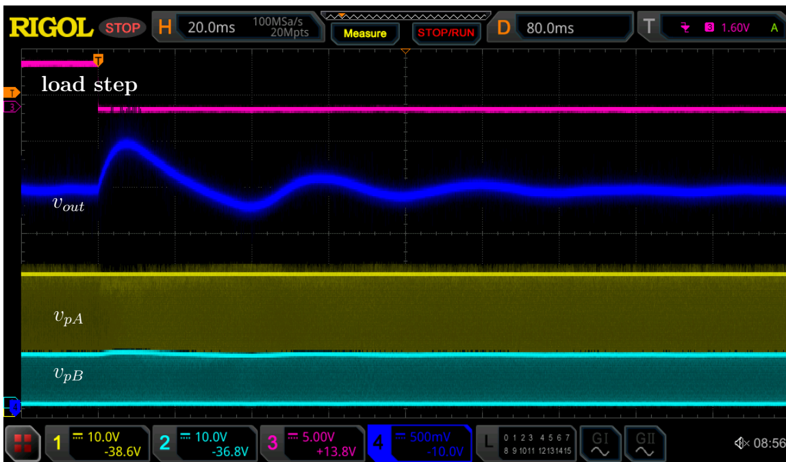
Figure 4-13: Experimental transient response to R_{load} step from 300\ \Omega to 600\ \Omega with V_{in} = 30\ \text{V} and V_{cmd} = 10.4\ \text{V} . The peak deviation from steady state is 600\ \text{mV} (5.8% of V_{cmd} ) and the 2% settling time is 18.4\ \text{ms} . Figure source: Joshua Piel.
