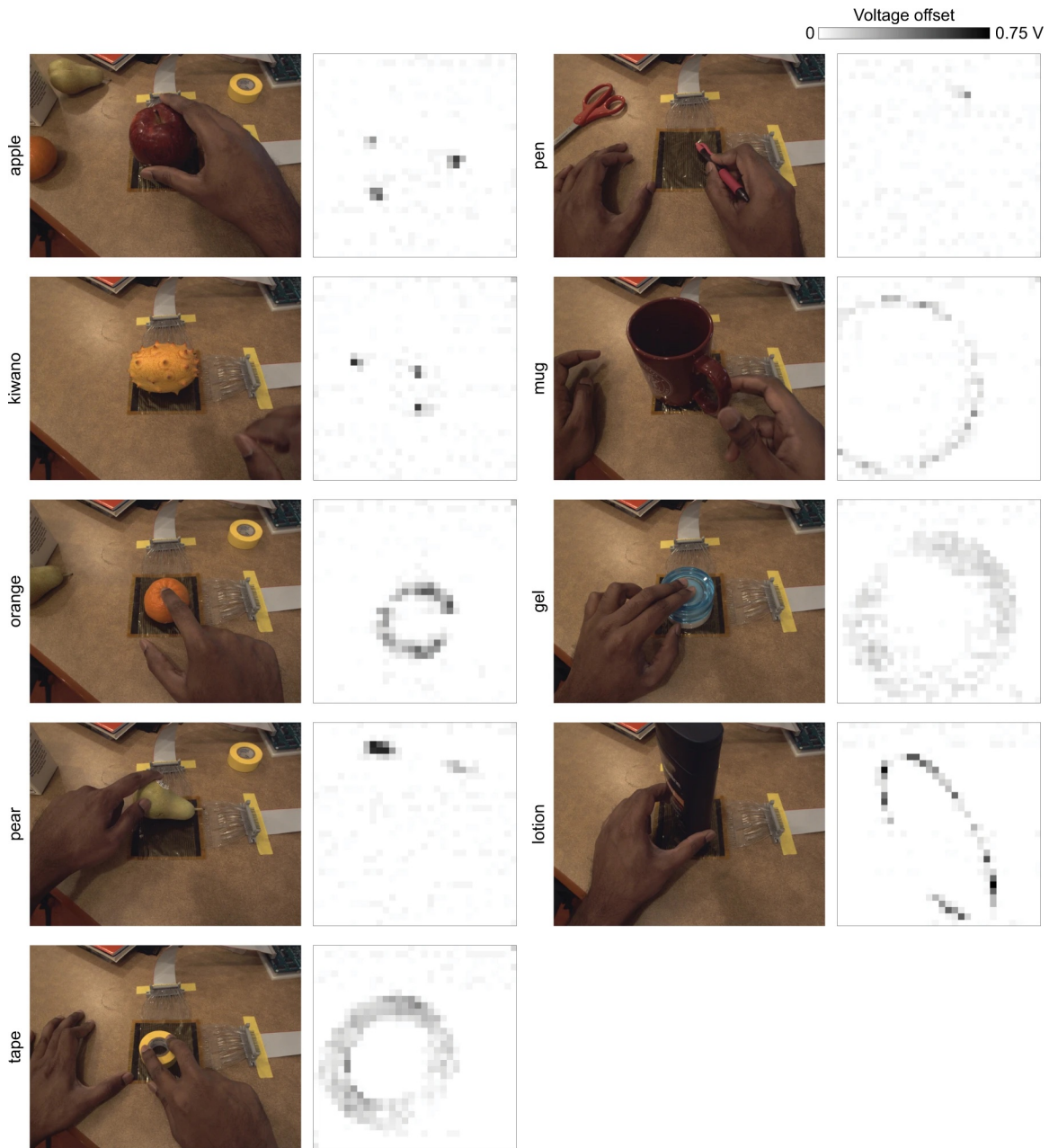
Figure 8-7: Sample recordings of nine objects on regular 32 \times 32 arrays on a flat surface. Nine different objects are manipulated on a regular sensor array (Figure 8-6d) placed on a flat surface. The resting patterns of these objects can be seen easily. Pressing the tactile array with sharp objects like a pen or the needles of a kiwano yields signals with a single sensor resolution.
