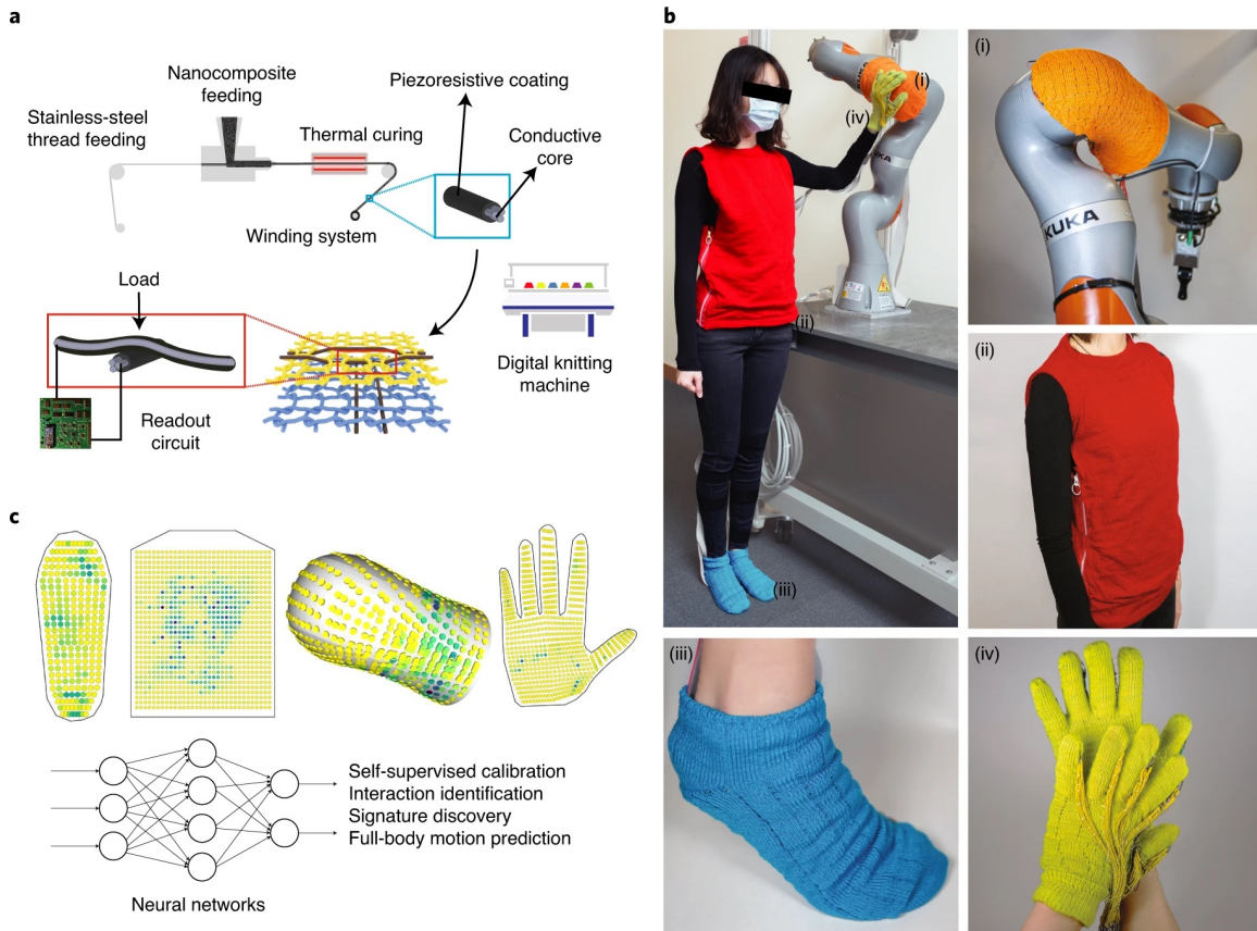
Figure 9-1: Textile-based tactile learning platform. (a) Schematic of the scalable manufacturing of tactile sensing textiles using a customized coaxial piezoresistive fibre fabrication system and digital machine knitting. A commercial conductive stainless-steel thread is coated with a piezoresistive nanocomposite (composed of polydimethylsiloxane (PDMS) elastomer as the matrix and graphite/copper nanoparticles as the conductive filler). (b) Digitally designed and automatically knitted full-sized tactile sensing wearables: (i) artificial robot skin, (ii) vest, (iii) sock and (iv) glove. (c) Examples of tactile frames collected during human–environment interactions and their applications explored using machine learning techniques.
