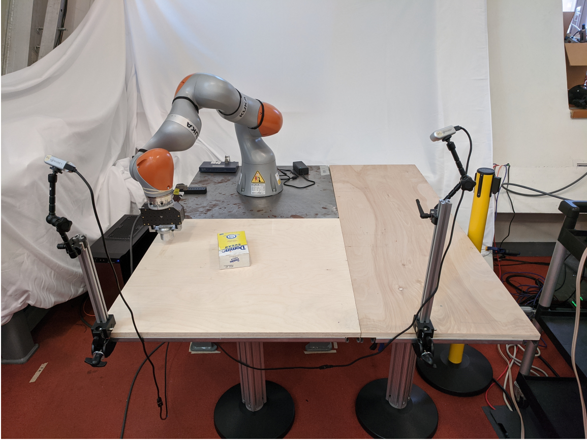
Figure A-1: Overview of our experimental setup. It includes two external Realsense D415 cameras. Images from both cameras are used to train the dense-descriptor model, while only the right camera is used at runtime to localize the keypoints on the object.
