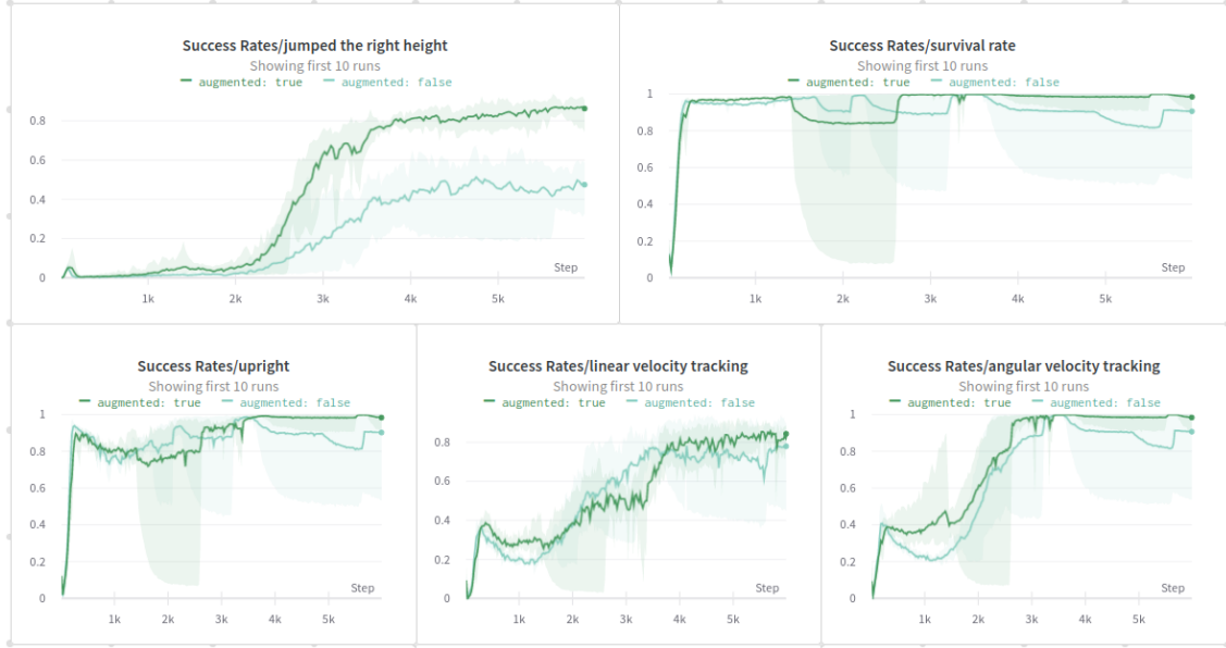
Figure 3-2: The results of training the Mini Cheetah simulated agent. Two average trends are shown with a central average line per iteration and a shaded region indicating the best and worst performing learning runs. The dark green curve represents learning runs with augmentations and the light blue line represents naively trained policy performance. It is not possible to compare convergence rates between the graphs since final performance differed, but augmented policy performance at jumping accurately was 1.75 times better the naively trained policies.
