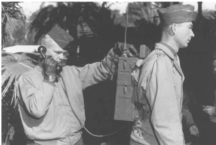
The SCR-300, better known as the walkie-talkie; below, radioman with handie-talkie (SCR-536) on Okinawa.
