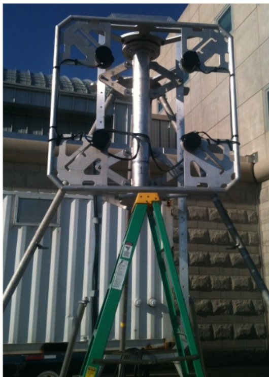
Figure 2.6: Photo of the square 75 cm array on one of the tripods of the scintillation system. Image by A. Lavery of WHOI.
