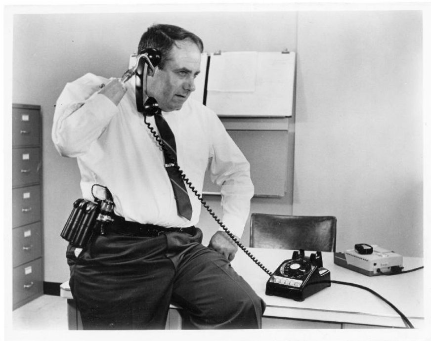
Figure 5. Man in a suit and tie using an early prototype of the Boston Arm to pick up the telephone. Collection on the Boston Arm (Boston Elbow), MIT Museum.
