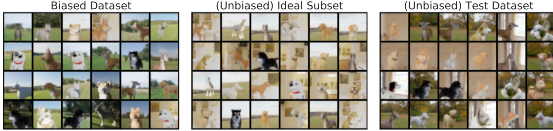
Figure C-1: The full 15k-image auxiliary dataset (Left) contains a background bias where dogs appear more frequently outdoors and cats appear more frequently indoors. We only show dog images here to highlight the background bias. The unbiased 3k-image subset (Middle) does not have any background bias. Training on the unbiased subset results in better test accuracy on the unbiased test set (Right), showing that more data is not always more helpful.
