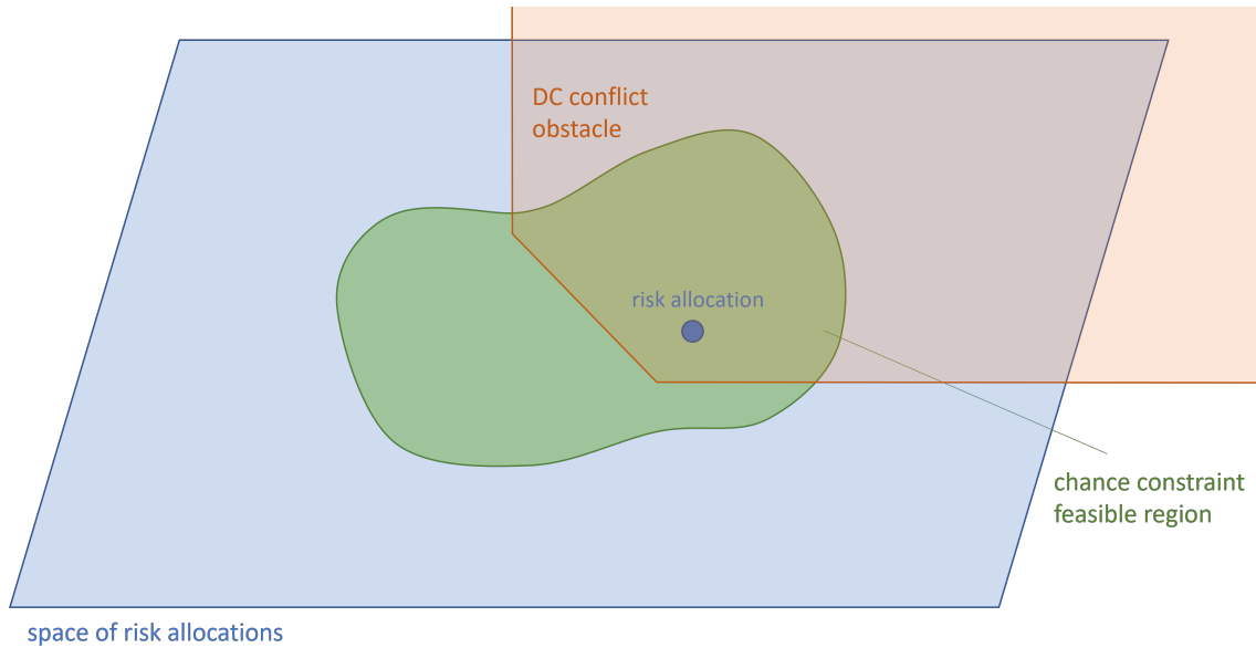
Figure 4-29: To satisfy the disjunctive linear constraint, one can view its negation as the obstacle in risk allocation space. The negation is exactly the intersection of all the hyperplane-bounded obstacles. Hence, it is a convex polytope obstacle.
