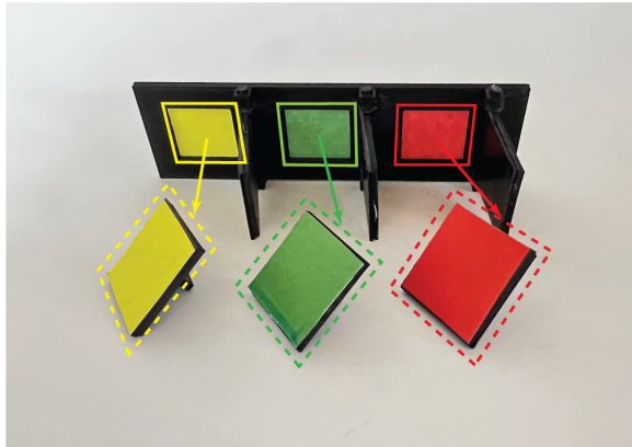
Figure 4: Selectively magnetic lock-and-key systems. Colored locks (solid lines) mate with keys of the associated color (dashed line), but not others.
