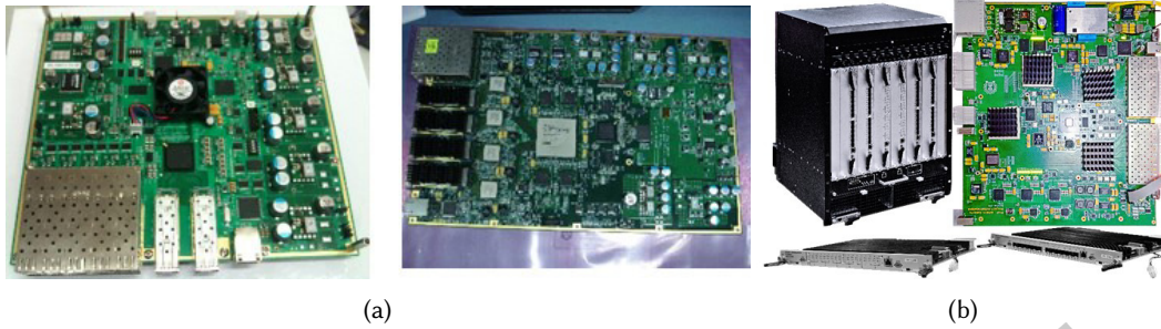
Fig. 9. a) The edge and regional SDN routers. b) The core SDN router. Chassis (above left), PCB (above right), the switching card (bottom left), the IO card (bottom right).
