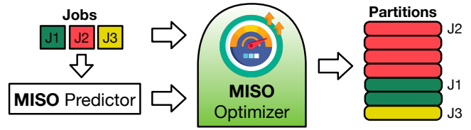
Figure 9: MISO optimizer to generate optimal MIG partition.
