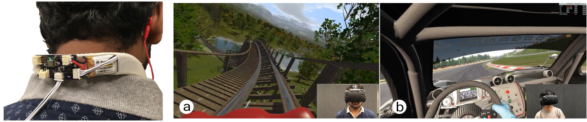
Figure 4: Left: The MoveU device as worn by a VR users with electrodes connected behind each ear for electrically stimulating the inner ear using galvanic vestibular stimulation (GVS). Right a,b): MoveU used in a VR roller coaster and VR car driving experience to match the sensory perception of riding a coaster and a car by stimulating the inner ear during turns.
