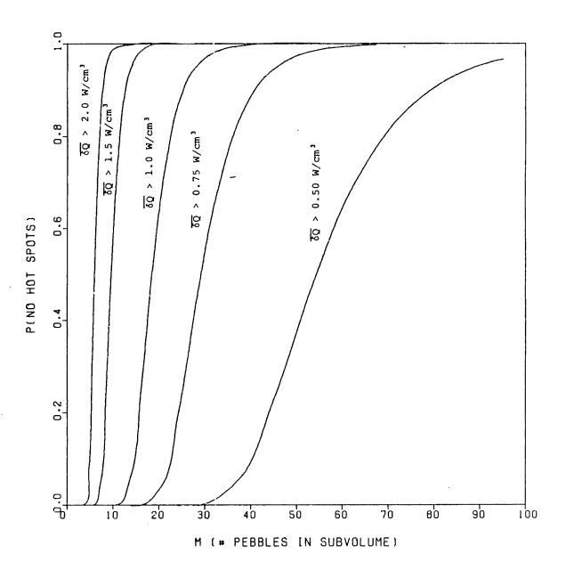
FIG. 4.19: Zero hot-spot probabilities for power density in the high power density zone of the 200 MWth HTR-Modul.
