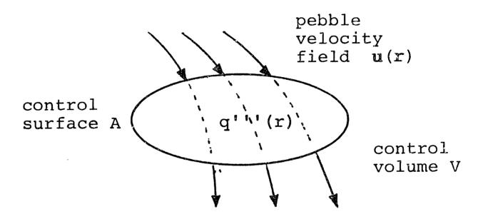
FIG. 3.14: Control volume for energy balance within the reactor.
