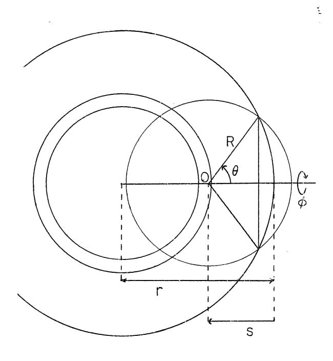
FIG. 6.17: Geometry for calculating fission product release due to direct recoil.
