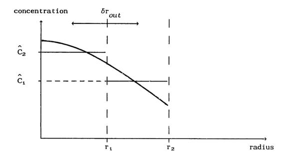
FIG. 6.8: Discrete and continuous fission product profiles in the innermost particle shells.
