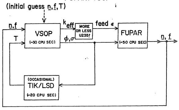
FIG. 4.13: A simple iterative scheme for FUPAR/VSOP.
