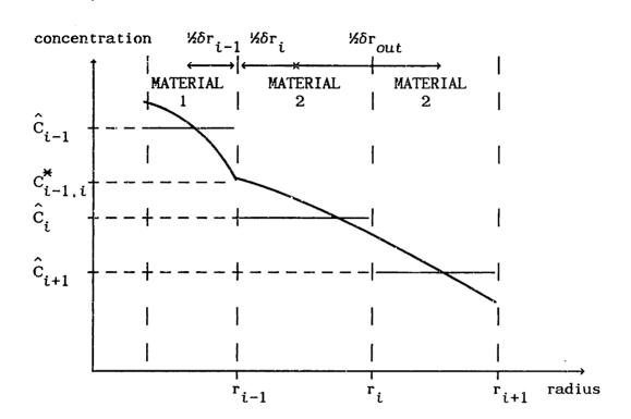
FIG. 6.14: Discrete and continuous fission product profiles near a shell with inner neighbor composed of a different material.
