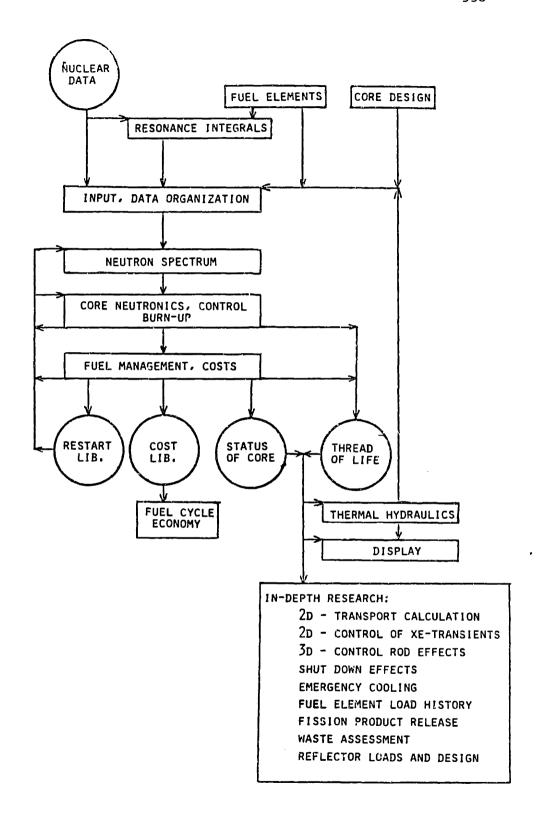
FIG. B.1a: Structure of the VSOP computer code: physics simulation [T2].
