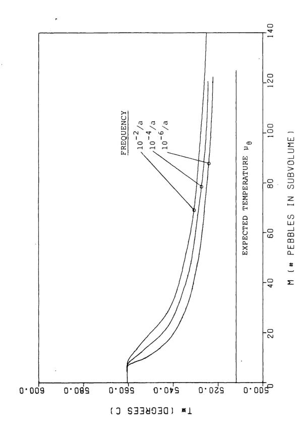
Maximum hot spot severities in the base core's highest power density region
