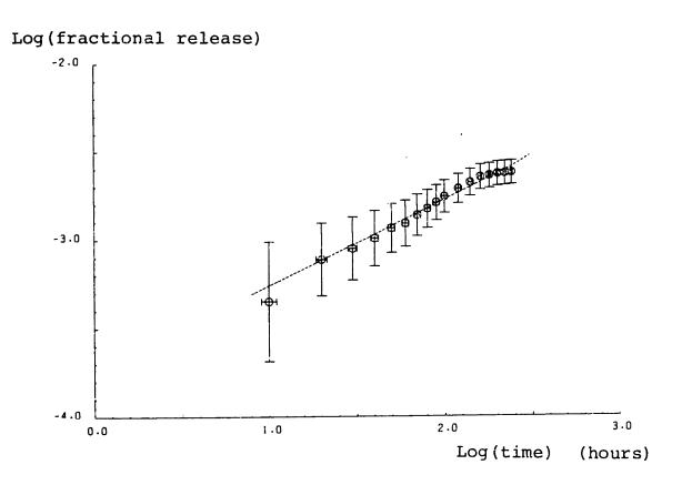
FIG. 6.1: Fission product release as a function of time during a post-irradiation annealing experiment [A3].
