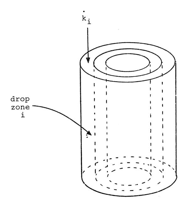
FIG. 3.6: Idealized pebble bed reactor with radial "drop zones."
