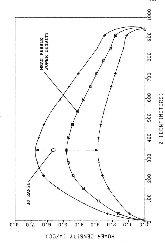
Axial power density and power density standard deviation distributions in the DCGT core. 5.27:
