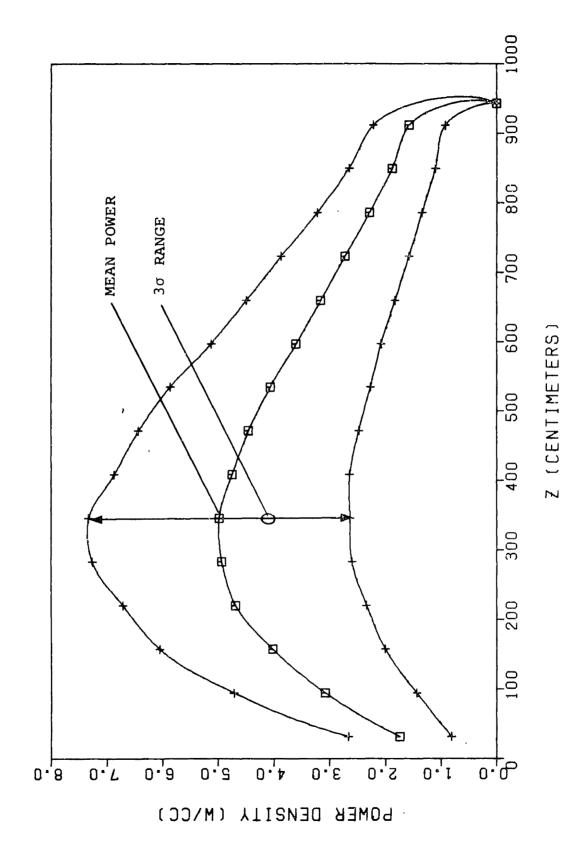
Axial power density and power density standard deviation distribution in the base core. 4.
