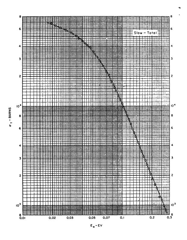
FIG. 5.14: Total neutron cross section for Gd-155 at thermal energies
