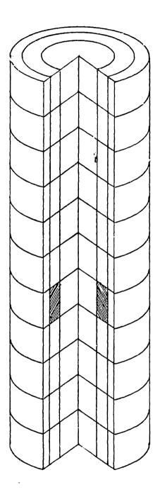
FIG. 4.3: An idealized pebble bed core divided into axial and radial regions.
