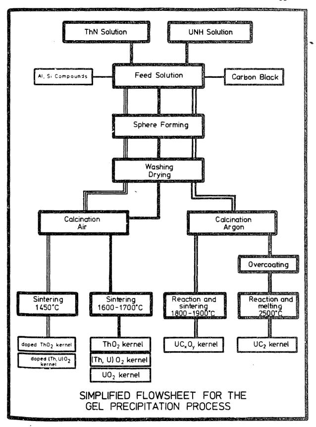
FIG. 2.3: The gel precipitation method for fuel kernel manufacture [K1].
