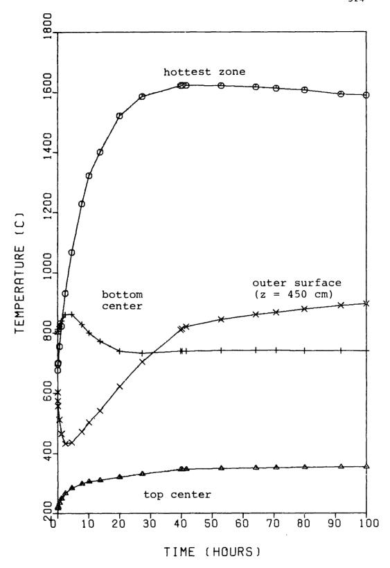
FIG. 5.25: Temperature behavior of the poisoned core following a postulated depressurization accident.
