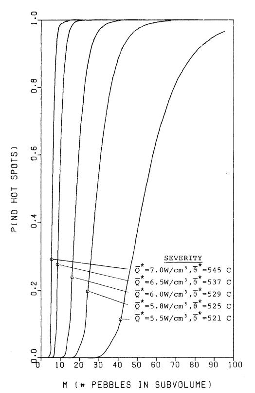
FIG. 5.9: Zero hot spot probabilities in the base core's high power density zone.
