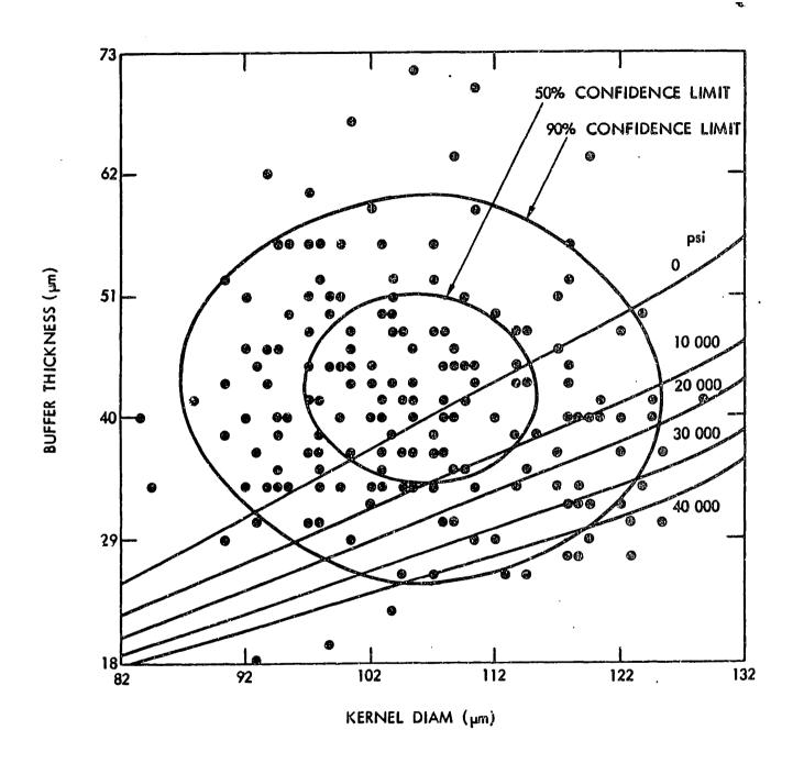
FIG. 2.5: Gulden's "direct method" for estimating pressure vessel failure fractions [G1].
