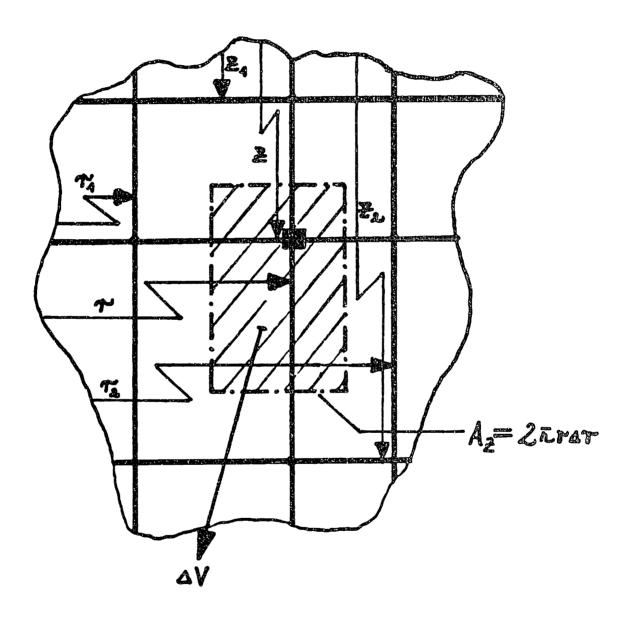
FIG. D.1: Finite difference mesh for heat conduction within the pebble bed [B6].
