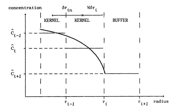
FIG. 6.10: Discrete and continuous fission product profiles near the inner buffer surface.
