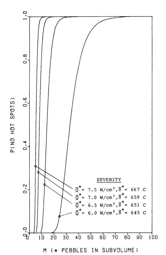
FIG. 5.22: Zero hot spot probabilities in the poisoned core's high power density zone.
