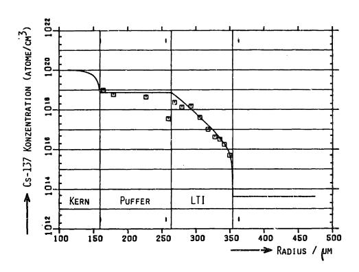
FIG. 6.9: Measured concentration profiles illustrating high buffer diffusivity [A3].
