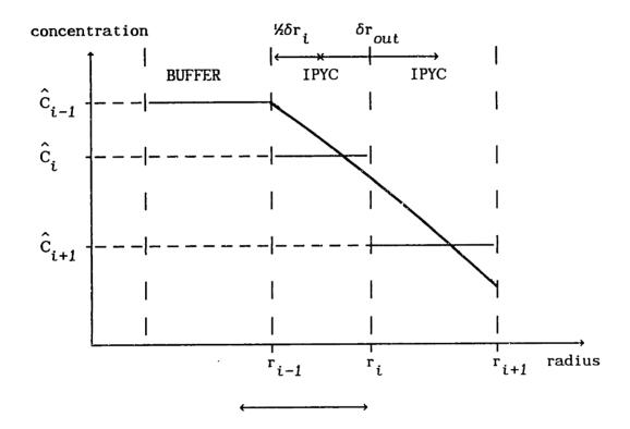
FIG. 6.11: Discrete and continuous fission product profiles in and adjacent to the buffer layer.
