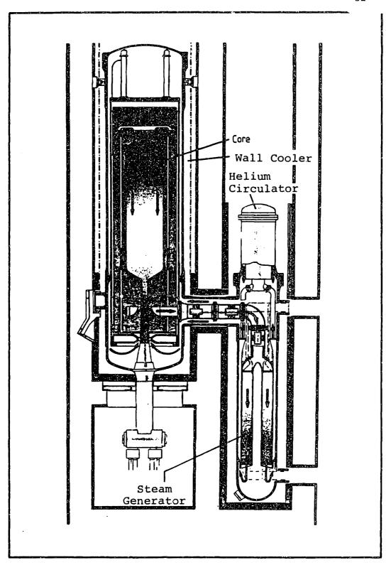
FIG. 1.2: The 200 MWth KWU/Interatom HTR-Modul.
