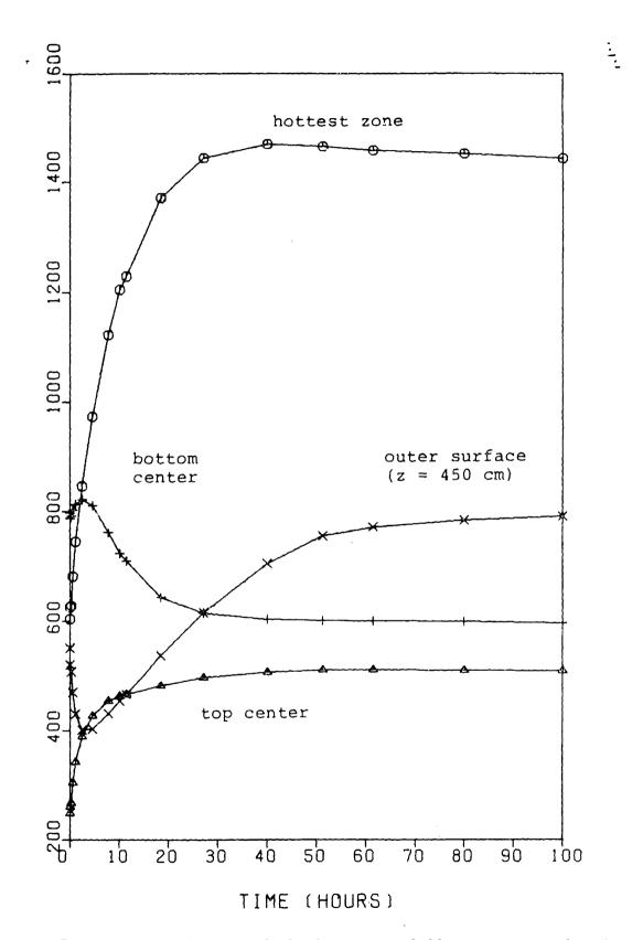
FIG. 8.10: Temperature behavior of the base core following a postulated depressurization accident.
