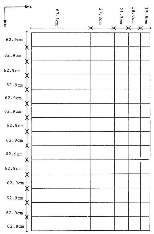
FIG. 5.1: Discretization used for reactor analysis.
