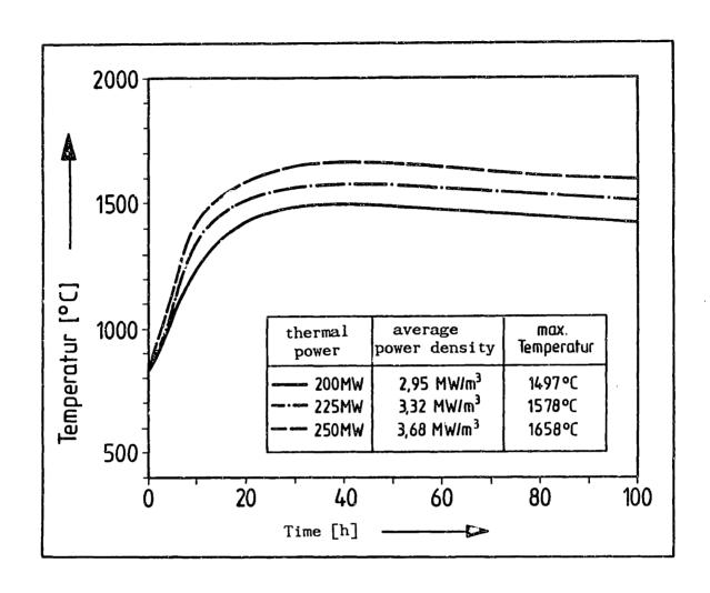
FIG. 2.14: Effects of reactor power density on maximum temperatures achived in core heatup accidents [J1].
