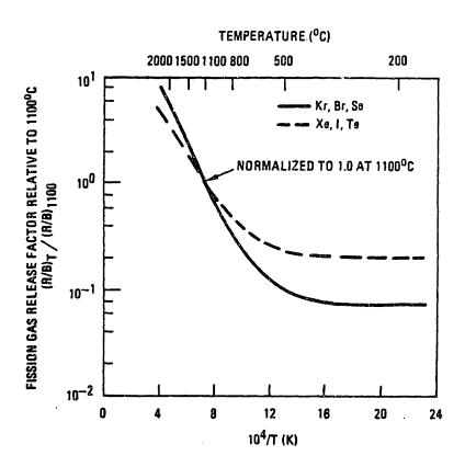
FIG. 2.10: R/B correlation for gaseous fission products generated in contamination granules [S2].
