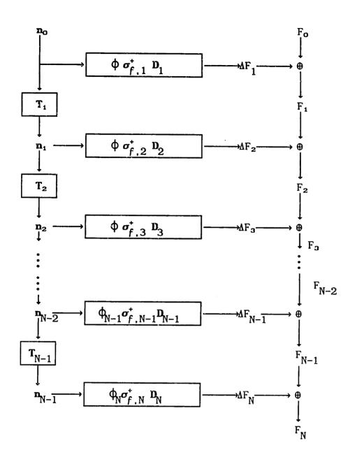
FIG. 4.5: Block diagram for collapsing the burnup transition matrices.
