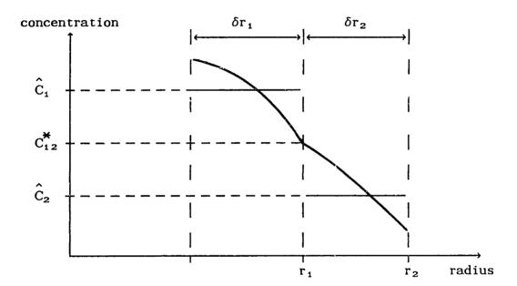
FIG. 6.12: Two adjacent spherical shells of differing materials.
