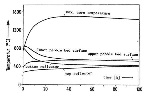
FIG. 2.13a: Temperature transient for loss of forced circulation, reactor under pressure (RuD) [J1].
