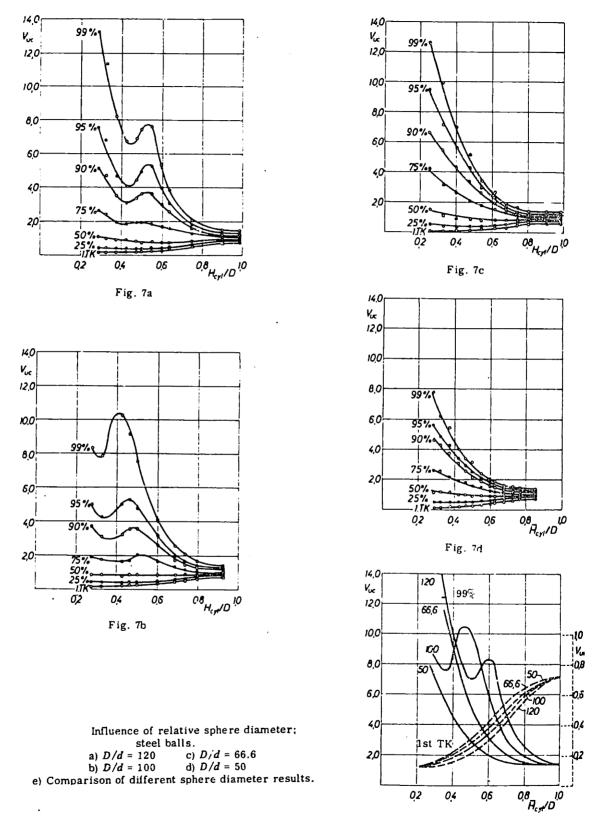
FIG. 3.5: Influence of reactor height/diameter (H/D) and pebble/core diameter (d/D) on test bed residence spectra [V1].
