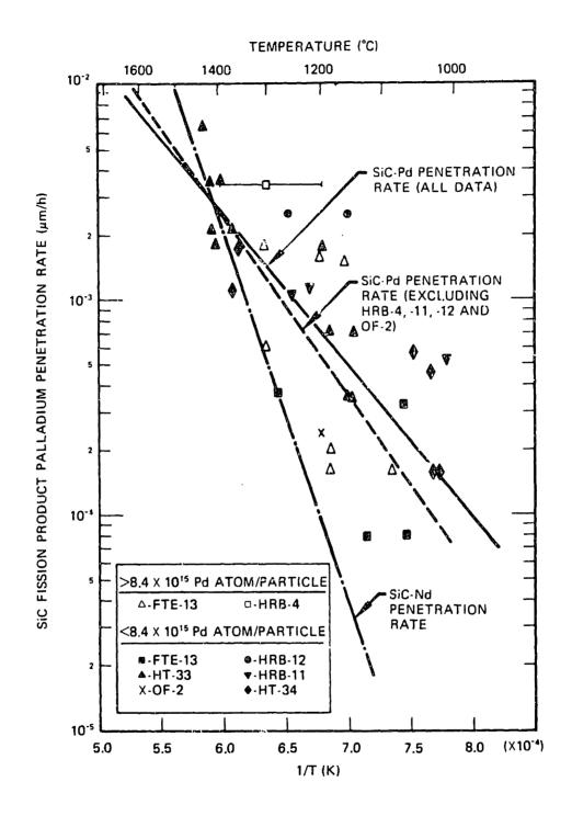
FIG. 2.8: Experimental corrosion rates indicating temperature dependence [T3].
