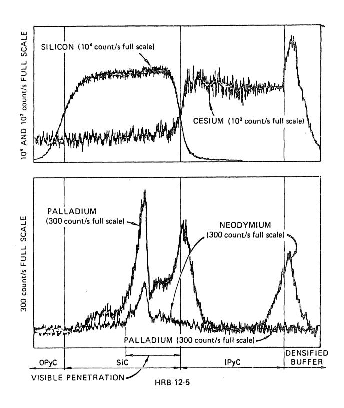
FIG. 2.7: Electron microprobe analysis of a SiC coating layer under corrosion attack by fission product palladium [T3].
