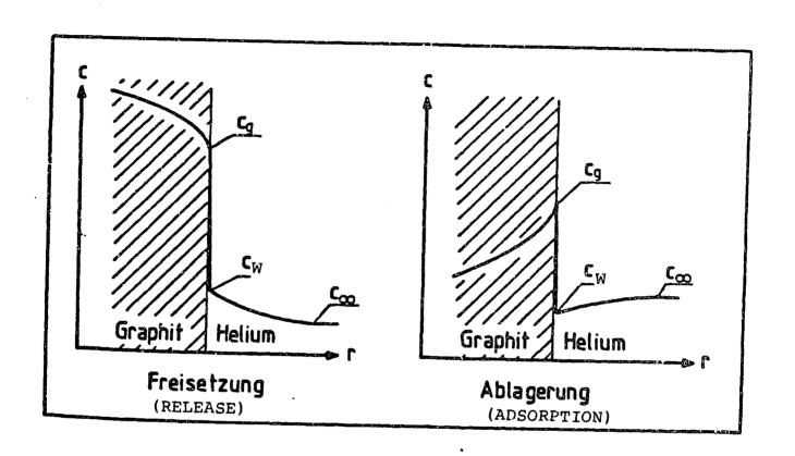
FIG. 6.19: Fission product release and adsorption on graphite surfaces.
