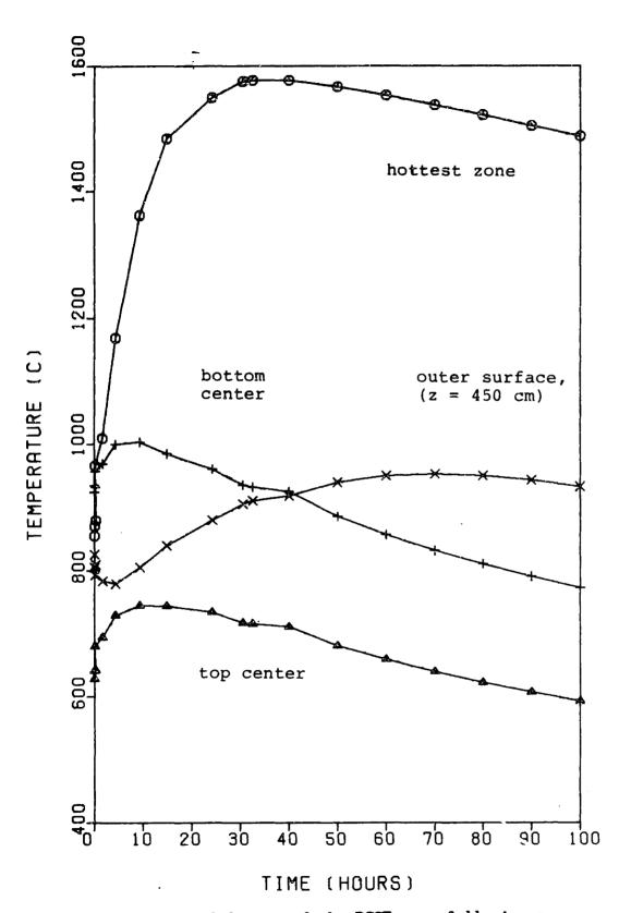
FIG. 5.35: Temperature behavior of the DOGT core following a postulated depressurization accident.
