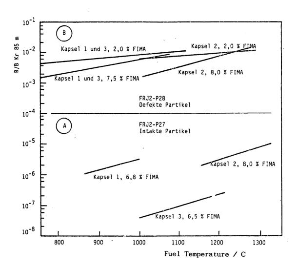
FIG. 2.11: In-core R/B measurements for failed and intact fuel particles [H2].
