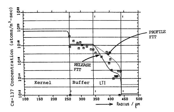
FIG. 6.3: Comparison of measured and predicted fission product profiles [A3].
