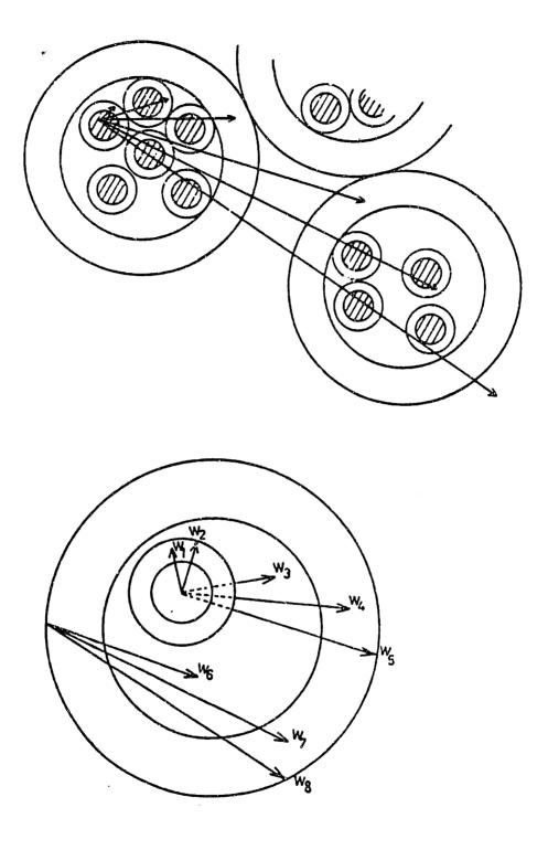
FIG. B.2: Neutron trajectories for doubly-heterogeneous escape probability calculations.
