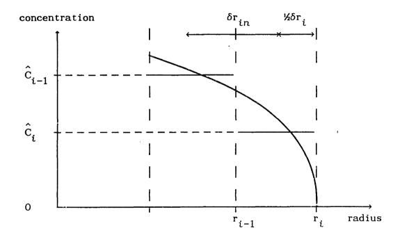
FIG. 6.15: Discrete and continuous fission product profiles near the outermost particle shell.
