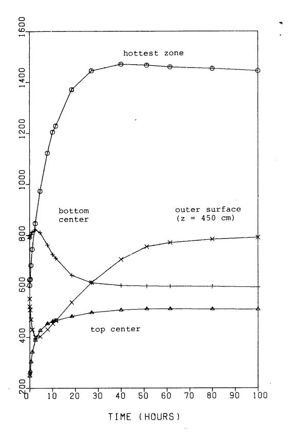
FIG. 5.13: Temperature behavior of the base core following a postulated depressurization accident.
