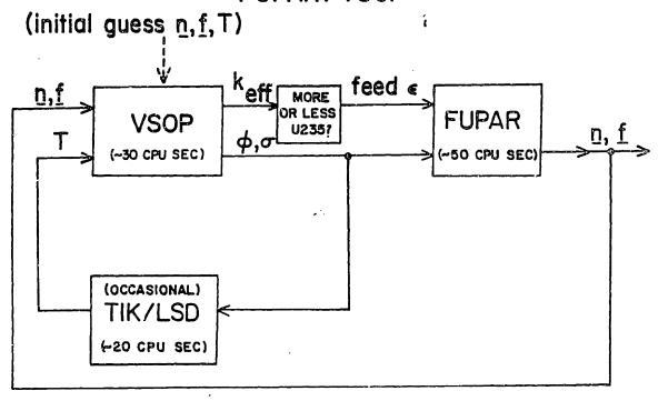
FIG. 8.4: A simple iterative scheme for FUPAR/VSOP.
