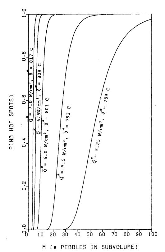
FIG. 5.32: Zero hot spot probabilities in the DOGT core's high power density zone.
