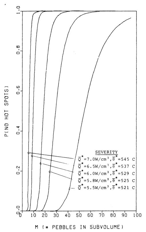
FIG. 8.7: Zero hot spot probabilities in the base core's high power density zone.
