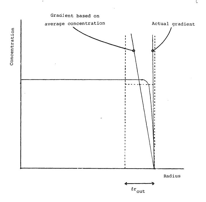
FIG. 6.16: Fission product concentration profile near the particle boundary at very short diffusion times.
