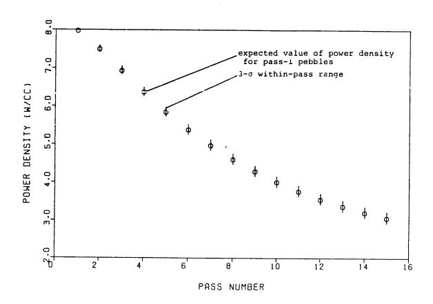
FIG. 5.6: Pass-dependent power densities and power density standard deviations in the high power zone of the base core.
