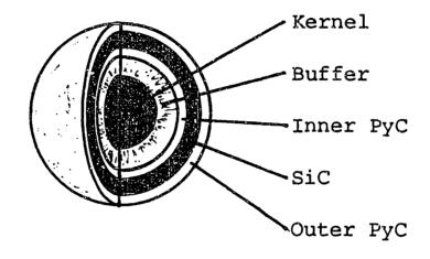
FIG. 2.1: The TRISO fuel particle design.
