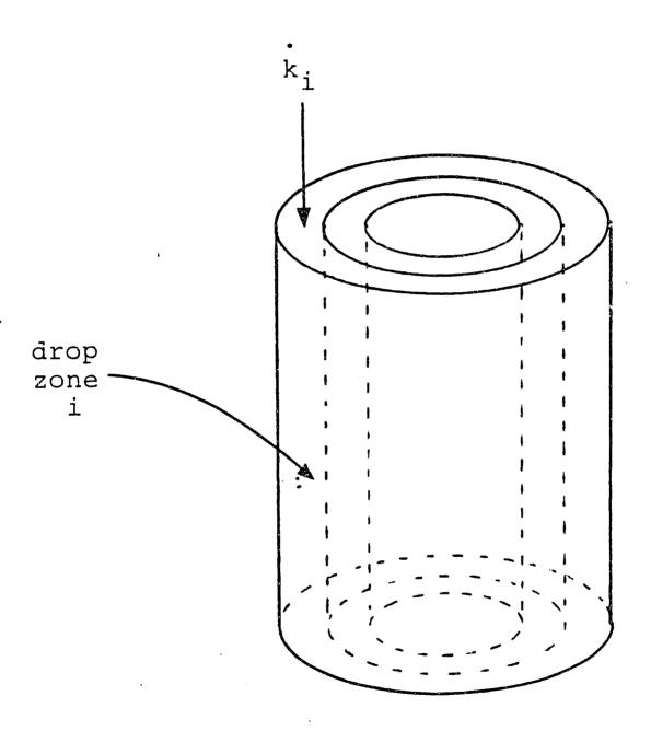
FIG. 8.3: Idealized pebble bed reactor with radial "drop zones."
