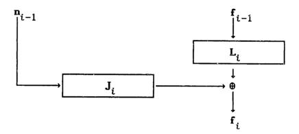
FIG. 4.6: Input/output diagram for fission product densities.
