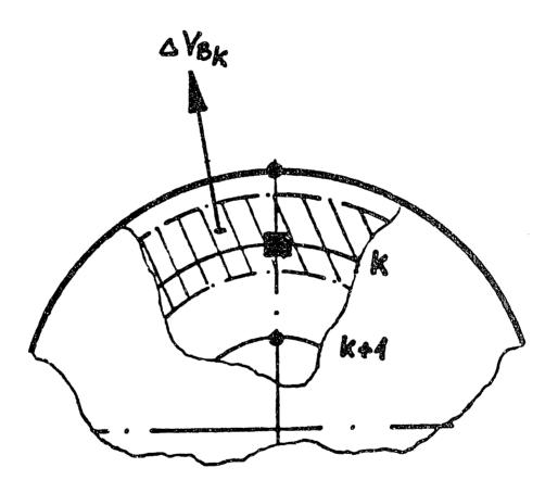
FIG. D.2: Finite difference mesh for heat conduction within a pebble fuel element [B6].
