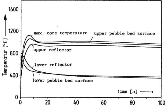
FIG. 2.13b: Temperature transient for loss of forced circulation, reactor depressurized (DES) [J1].
