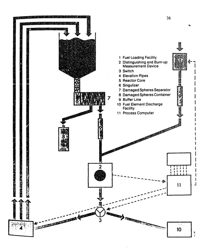
FIG. 1.3: A pebble-bed reactor refueling system.
