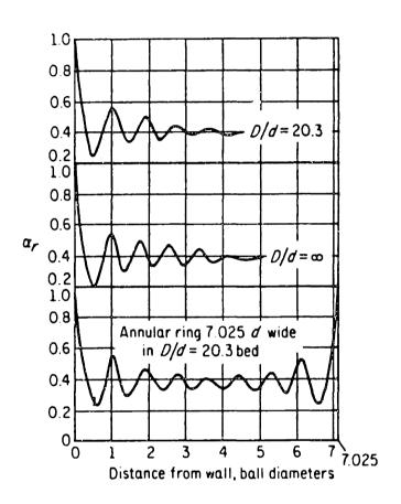
FIG. 3.1: Void fractions measured in scale model pebble beds [E1].
