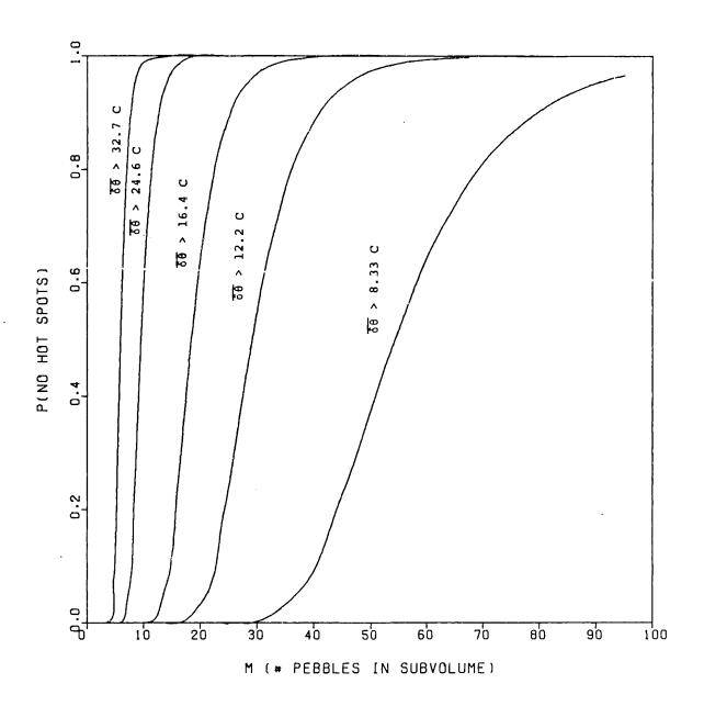
FIG. 4.20: Zero hot-spot probabilities for temperature in the high power density zone of the 200 MWth HTR-Modul.
