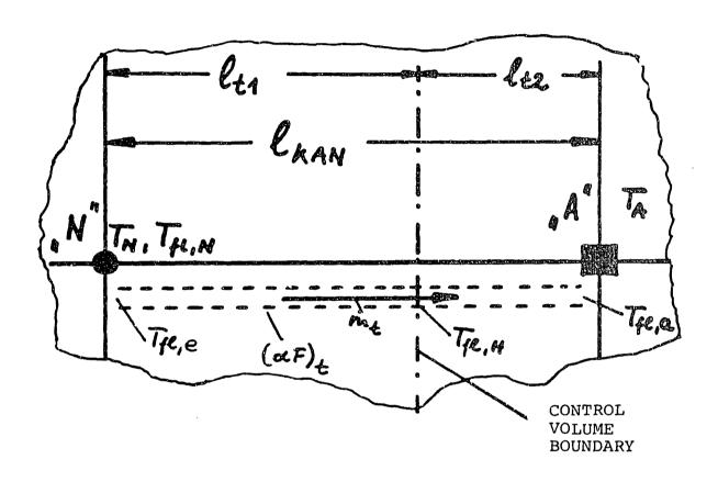
FIG. D.4: Partial channel for calculating gas temperatures [B6].
