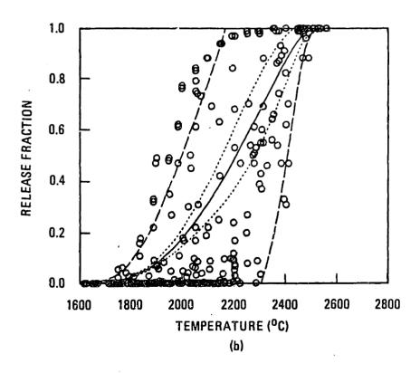
FIG. 2.12: Fuel particle failure rates measured in core heatup simulation tests [G5]
