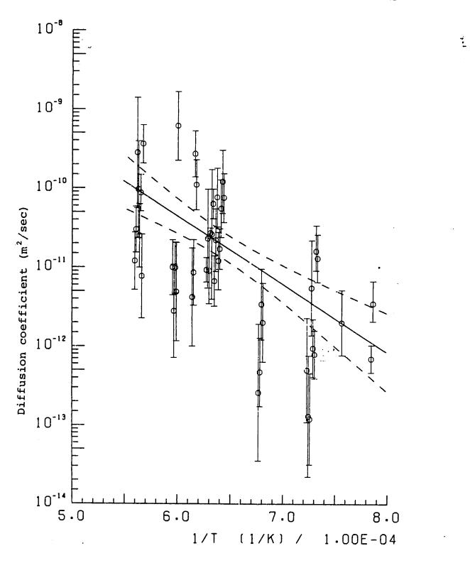
FIG. 6.2: Temperature dependence of R-fit diffusivities [A3].
