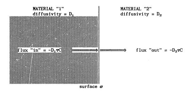
FIG. 6.5: Continuity of mass flux at a boundary between two different materials.
