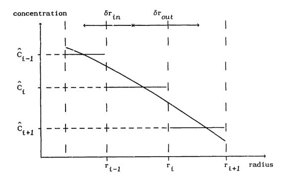
FIG. 6.7: Three adjacent spherical shells with identical materials.
