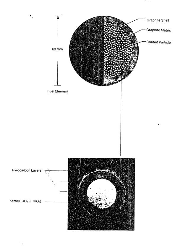
FIG. 8.1: An HTGR coated fuel particle and fuel element.
