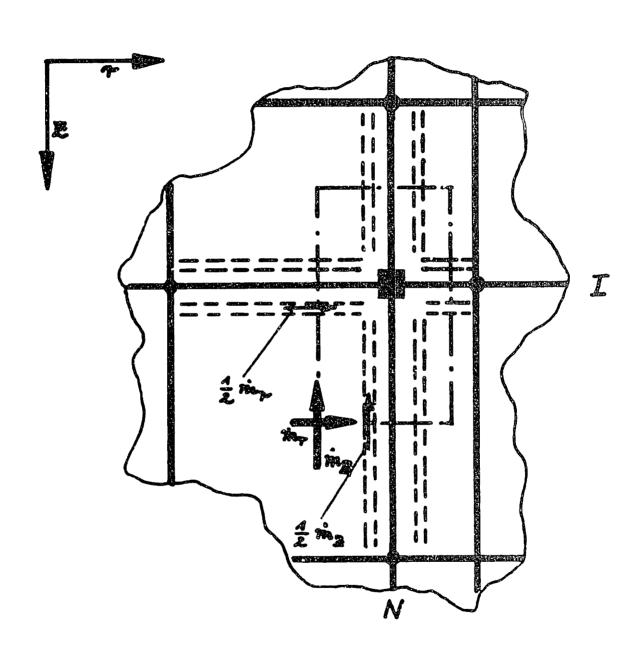
FIG. D.3: Coarse mesh for calculating gas temperatures in KONVEK [B6].
