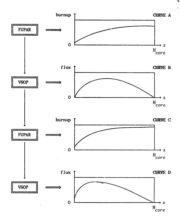
FIG. 4.14: Potential instability using FUPAR/VSOP to analyze few-pass cores.
