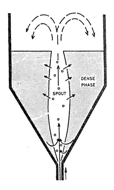
FIG. 2.4: Schematic diagram of a fuel particle coating furnace.
