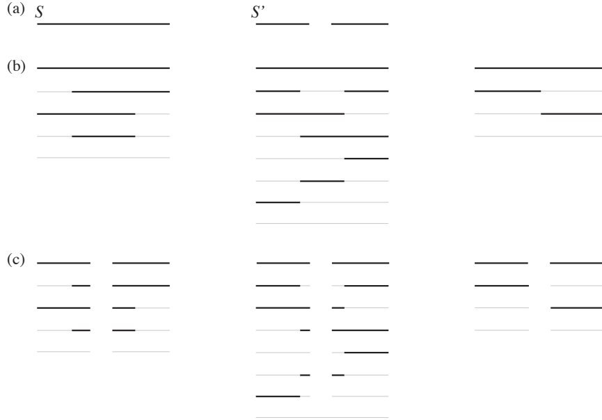
Figure 24. (a) A shape S made of a single line and a shape S' obtained by removing a part from S . (b) Three topologies for S . S is topologically connected only with the first topology. (c) Three subshape topologies for S' (treating S' as a part of S ). S' is topologically disconnected with the second and third subshape topologies.
