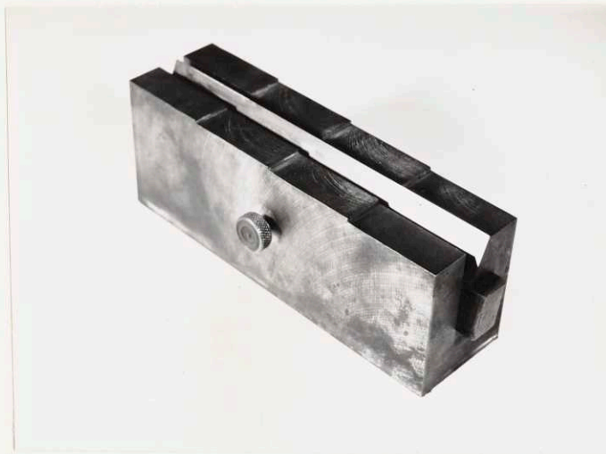
Fig. 3 - Close-up View of Knife in Holder
