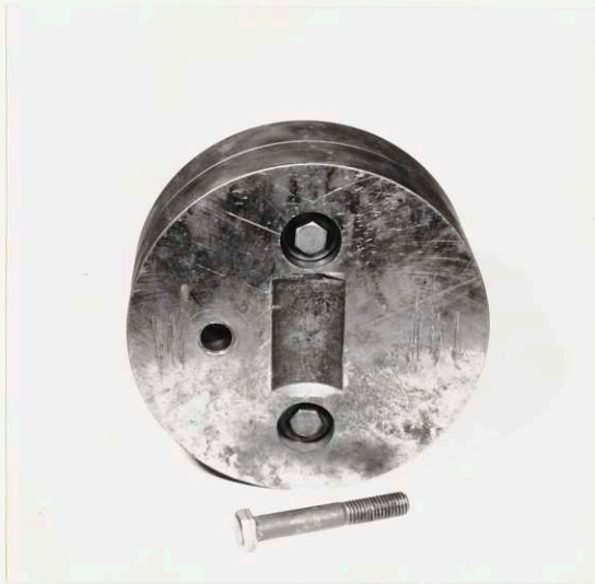
Fig. 7 - Bottom View of Loading Plate with Fixing Bolt
