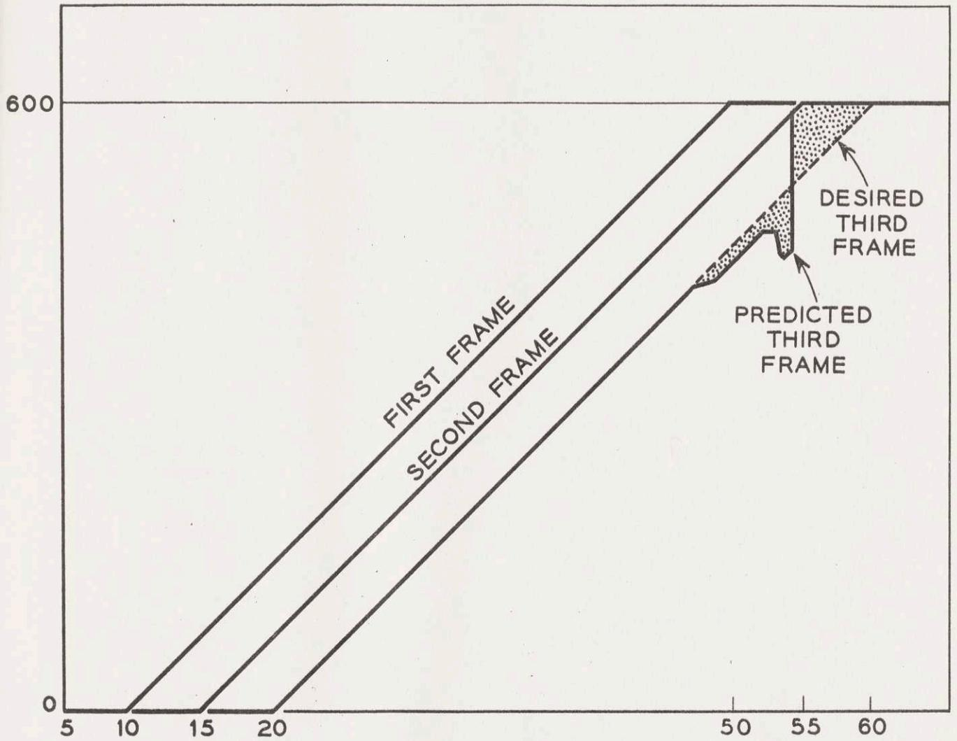
FIG. 3 EFFECT OF FIRST ORDER EXTRAPOLATION ON A DISPLACED RAMP
