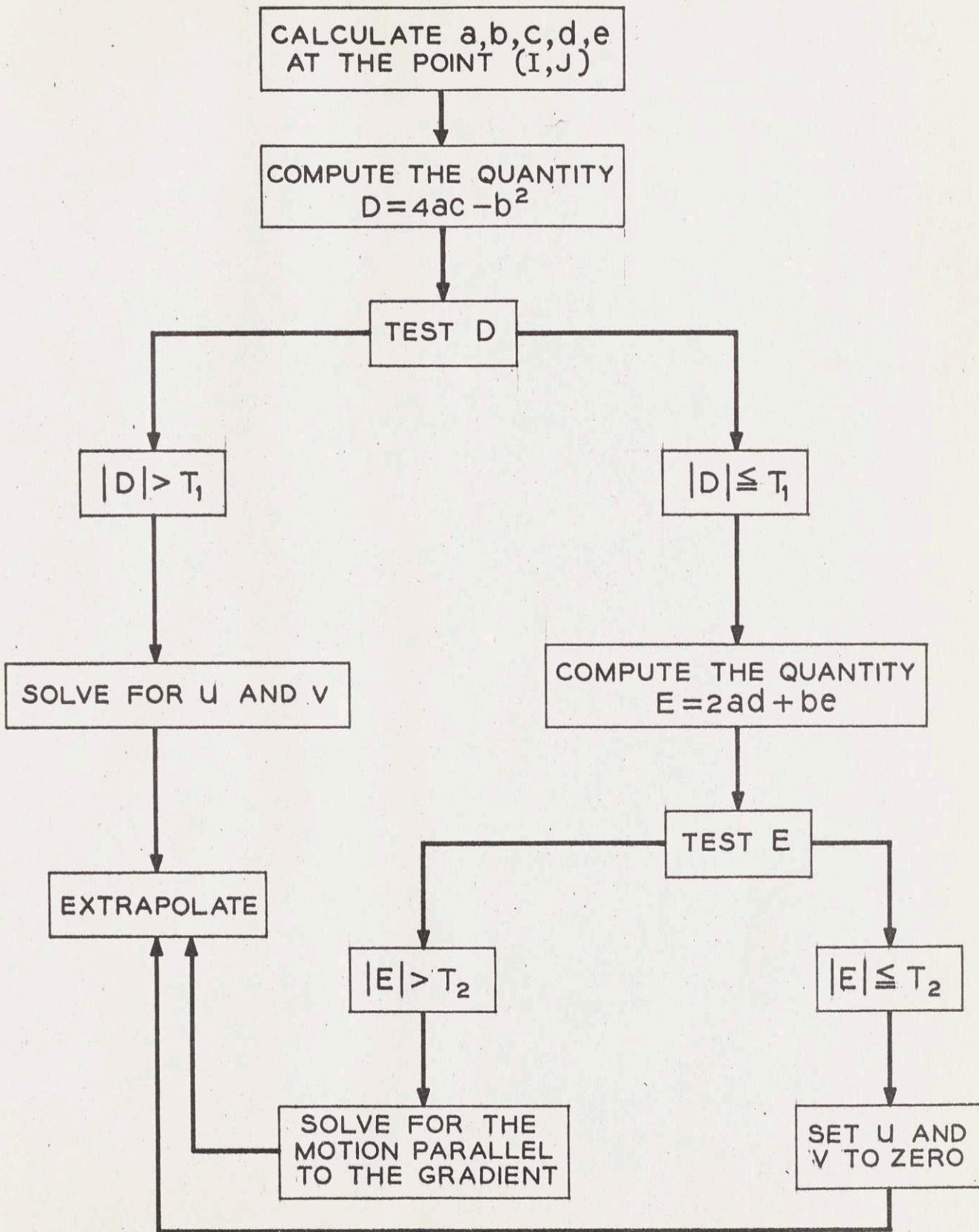
FIG 4 FLOW CHART FOR SECOND ORDER WITH  $h_1 = k_2 = 1, h_2 = k_1 = 0$
