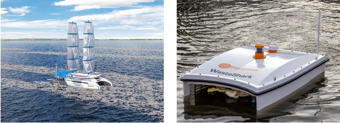
Figure 2-3: (Left) The Manta, a vessel being developed by SeaCleaners, for actively harvesting plastic waste pollution (The SeaCleaners, n.d.). (Right) An autonomous surface vessel called the Wasteshark, developed by Ranmarine Technology, designed for removing floating debris, including plastics, from marine environments (RanMarine Technology, 2021).
