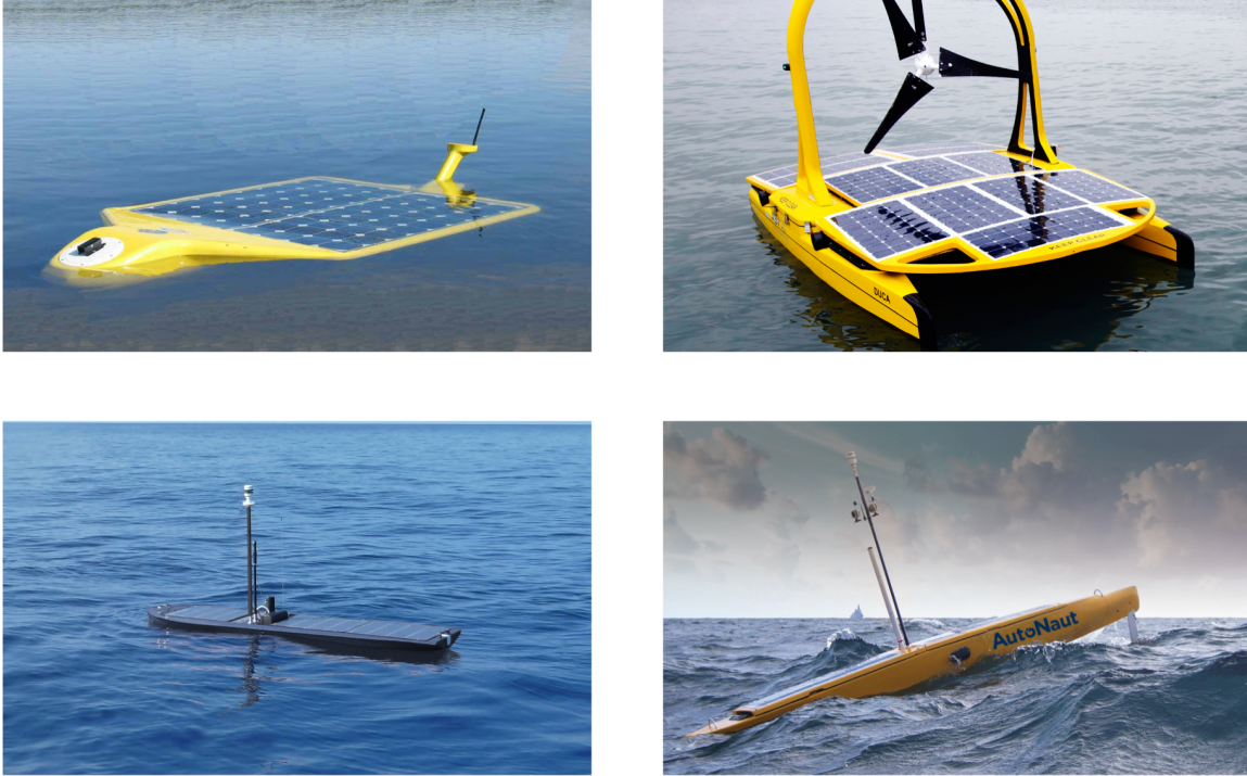
Figure 2-2: Examples of various autonomous marine vehicles equipped with energy harvesting capabilities. (Top left) The SAUV (Bekey et al., 2006). (Top right) The C-Enduro (Unmanned Marine Systems, 2013). (Bottom left) The Wave Glider (Coxworth, 2013). (Bottom right) The AutoNaut (Ocean News and Technology, 2019).
