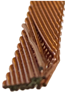
Figure 4-7: Photo of a 19 strand Litz bundle that was ultimately selected for the final machine.
