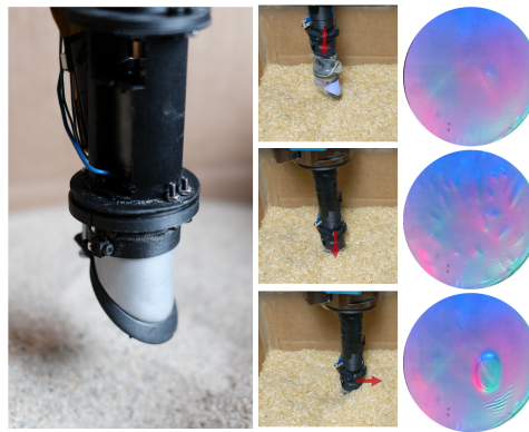
Fig. 1: Left : Digger Finger. Middle : Penetration motion. Right : Tactile data showing zero contact, granular media (rice), and object contact
