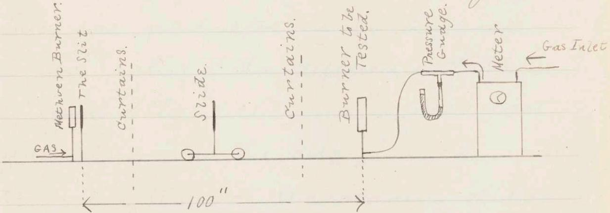
Before making a test I cleaned the chimneys and allowed the Methuen burner to come to its normal rate of burning and adjusted the height
