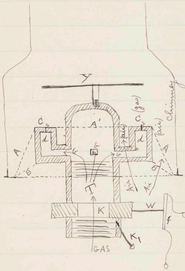
This sketch is a cross section of the burner. The gas enters as shown by the arrow, through the valve K, which is moved by the arm W and the lever f. The gas passes into the space T, and from here it passes through the three pipes marked b b b. These pipes lead into an annular space d. The gas passes from d through the holes s to the flame.
