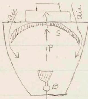
B is a common fish-tail burner (bulbed shaped) which is placed in this globe. No air can get in at the bottom. The products of combustion pass up & through the chimney. On the way they heat the porcelain plate S. The air for combustion comes in as marked and is heated by the porcelain plate. This heating of the air causes the combustion to be better and the illuminating power is increased.
