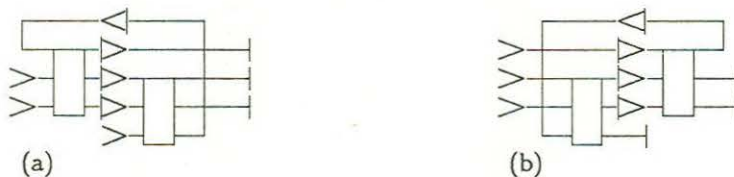
FIG. 7.1 (a) A conservative-logic network and (b) its inverse.
