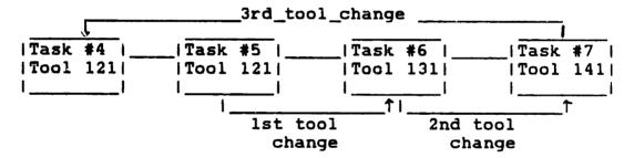
Tool change time for resource 1 is 2 seconds. Transport time for resource 1 is 2 seconds. Since the 3rd tool change occurs during the station to station move time, this tool change is not added to the total tool change time. Total tool change time is 4 seconds for this example.
