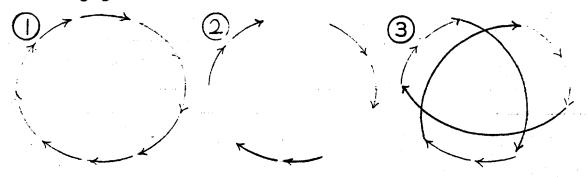
At this point, the algorithm compares the new cycle's length with the initial cycle's. If the length decreased, the new cycle becomes the shortest cycle yet found. If not, the initial cycle remains the shortest cycle yet found, and the algorithm marks the set of three edges to tell future iterations that deleting these edges will not lead to a shorter cycle.
