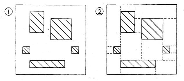
The following shows a chip's channel edges as dotted lines.
