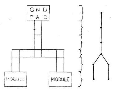
This notion of a node is compatible with the idea of making a horizontal cut. One way to determine the current flow through a node is to delete the node and find the total current of the tree fragment that has just been disconnected from the pad. Since a node can be a horizontal row of rectangles, this corresponds to the notion of cutting the tree by a horizontal line that runs through the rectangles and asking how much current flows across that line.
