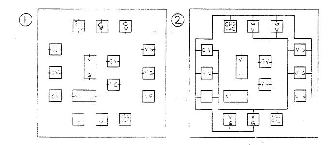
6.4.2. Constructing the trees sequentially to connect the logic modules
