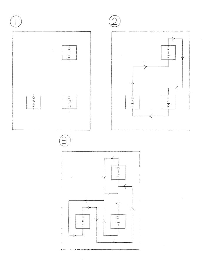
The cycle in the third figure is longer and less desirable than that in the second. This example shows that laying one edge's wires could block a path that would provide a short routing for a later edge. This later edge's routing may require long wires to avoid previously laid wires.
