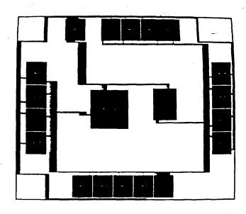
The resizer then stretches the wires in the y direction, resulting in the final layout of power-ground wires.
