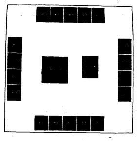
The power-ground phase uses the algorithm of Section 6.4.1 to lay a GND ring outside the pads and a VDD ring inside the pads, producing the following layout:
