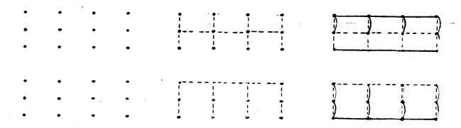
The next two sections describe two algorithms derived from this one. The first algorithm successively reroutes the trees' branches so as to shorten the trees' combined length. The second algorithm provides a different way to connect the second net's connection points after the first tree is complete. Instead of growing one tree for the second net, this algorithm grows several trees from several roots. PI's power-ground algorithm, described in Section 6.4, includes a version of this technique.
