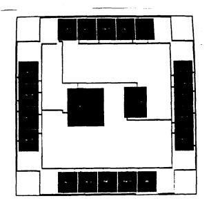
The power-ground phase uses the algorithm of Section 7 to determine how much current flows through each power-ground wire and how wide it has to be to handle this current. PI's resizer first stretches each power-ground wires to its appropriate width in the x direction.
