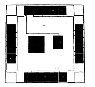
The power-ground phase uses the algorithm of Section 6.4.2 to lay branches from the VDD ring to the logic modules' terminals. The branches grow so that they do not cross the branches of the GND tree.
