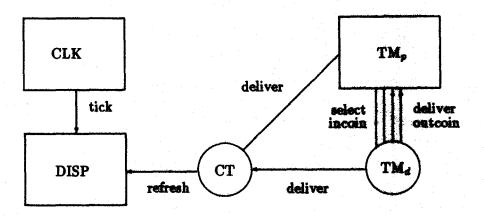
Figure 3.2: Ticket machine with display updated by clock
