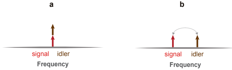
Figure 2-5. | Single-mode vs. two-mode. a. We define “single-mode” when the two modes, signal and idler, are degenerate. b. When the signal and idler are non-degenerate, we have “two-mode”.
