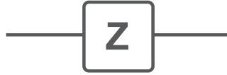
Figure 3-10. | Quantum Z gate. The quantum Z gate rotates the qubit state by \pi radian about z-axis.
