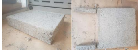
Figure 14: Photos of V2 molds after pouring (upper) and after curing (lower). The front plate part broke during removal.
