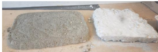
Figure 13: 1:2:2 volumetric ratio of cement, sand, gravel (left) and 1:2:4 volumetric ratio cement, sand, gravel (right).
