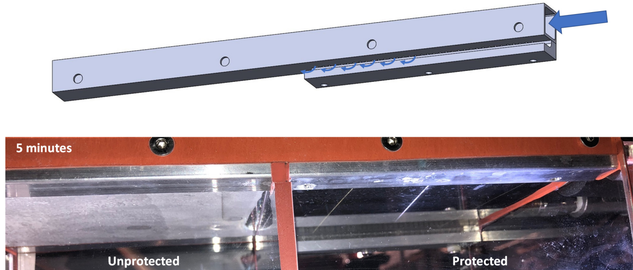
Figure 51 – Final nozzle geometry configuration (top) and example experiment showing the proxy SNGC efficacy after 5 minutes with a flow velocity of 2.5 m/s (bottom).
