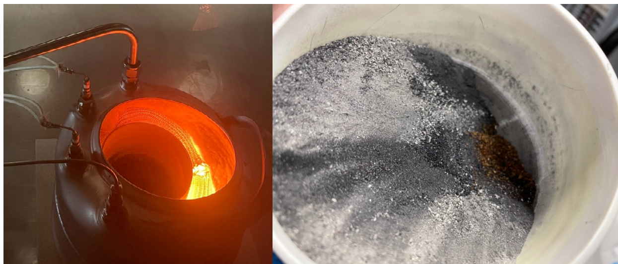
Figure 21 – Zirconium metal oxygen getter. Powdered metal heated in a zirconia crucible to >300\text{ }^{\circ}\text{C} to accelerate oxidation kinetics. Partially consumed getter material appears different colors as it oxidizes.
