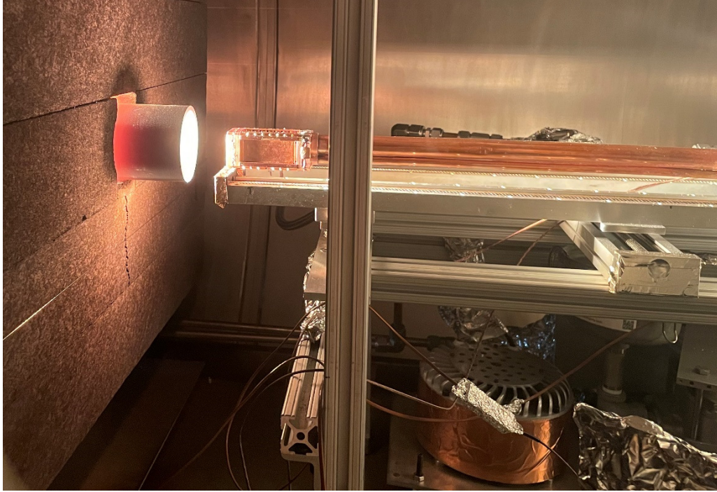
Figure 86 – Addition of a graphite tube emitter to fully shield from insulation contamination and accelerate measured deposition material.
