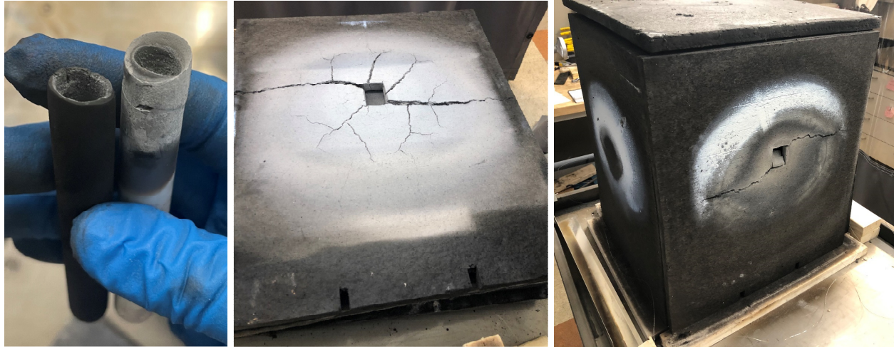
Figure 18 – Degraded oxide materials from high-temperature experimentation. In environments with very low oxygen content, oxides more readily reduce and often fall short of their rated operating temperatures. Contact between graphite and alumina tube (left) has eaten away both materials due to this accelerated decomposition. Alumina silicate boards (middle, right) show breakdown of structure and chemistry due to the reduced operating temperatures in the presence of carbon.
