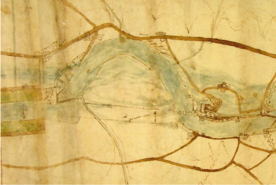
Figure 2: Girolamo di Pace, map and design of the Arno River upstream and downstream of Florence, sheet 4, 1534–1558, detail showing his proposed channel cut from the Rovezzano weir to the Girone mill, BRP, Carta Fiume Arno
