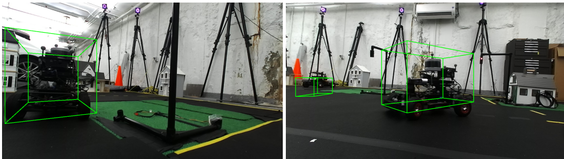
Figure 10-3: Ground truth bounding boxes (green) are automatically generated from the MiniCity's external motion capture system. Ground truth bounding boxes can be used for detector training, algorithm evaluation, and isolating downstream performance.
