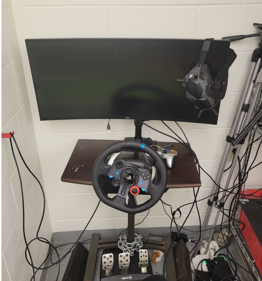
Figure 8-5: Manual Control Setup. A Logitech gaming steering wheel and pedals provides steering and acceleration inputs to the cars. First-person-view is streamed to either DJI FPV goggles or an external monitor for a view from the car's driver seat.
