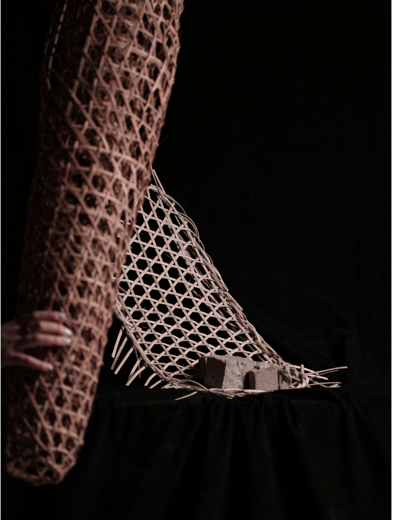
Fig 26. Triaxially woven sliced palm tree fronds and rattan
