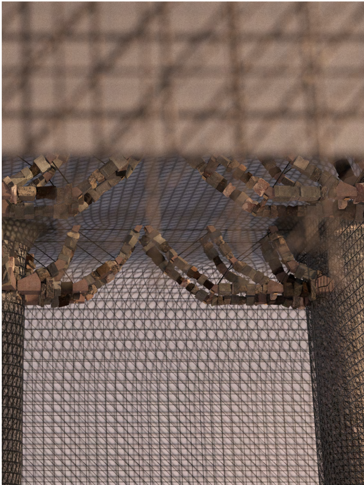
Fig 52. Rubble filled carbon fiber columns holding down the light roof hovering over the water.
