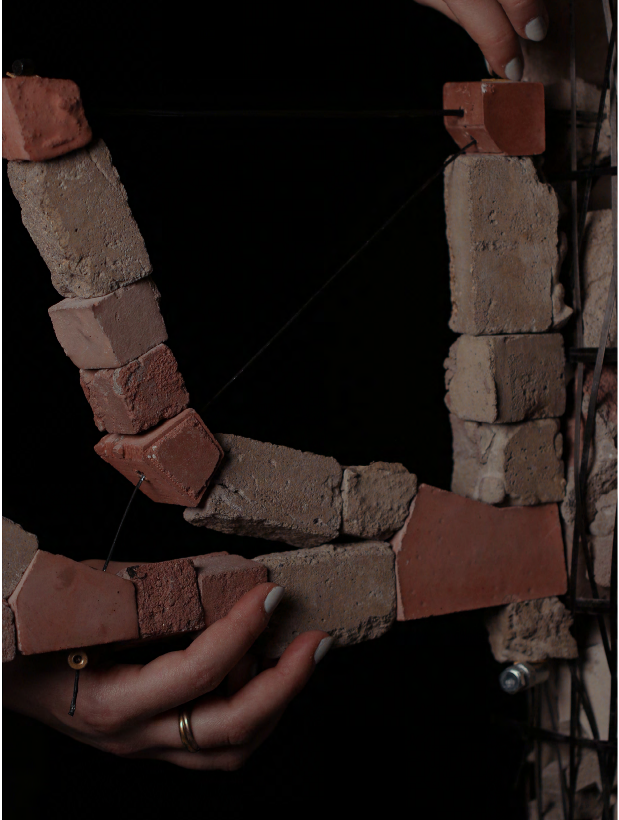
Fig 71. Close up of Joints Orienting the Rubble in the Planned Directions to Form the Overall Truss Topology.
