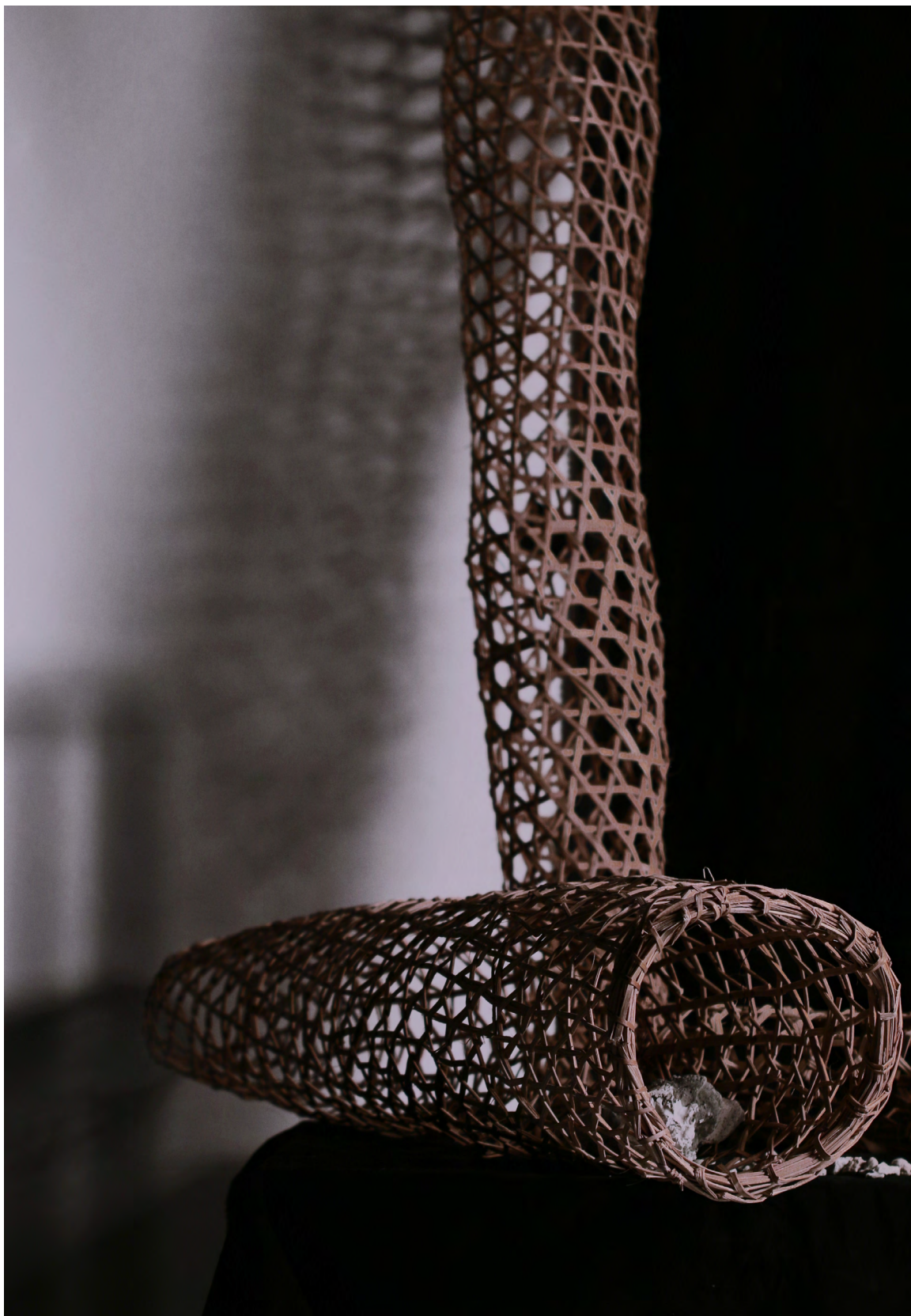
Fig 65. Woven Column Prototypes. Those palm fiber columns were woven by the craftsman, Muntathar, in the last third of thesis semester. They were used for comparison to the technique and results I achieved weaving the carbon fiber.
