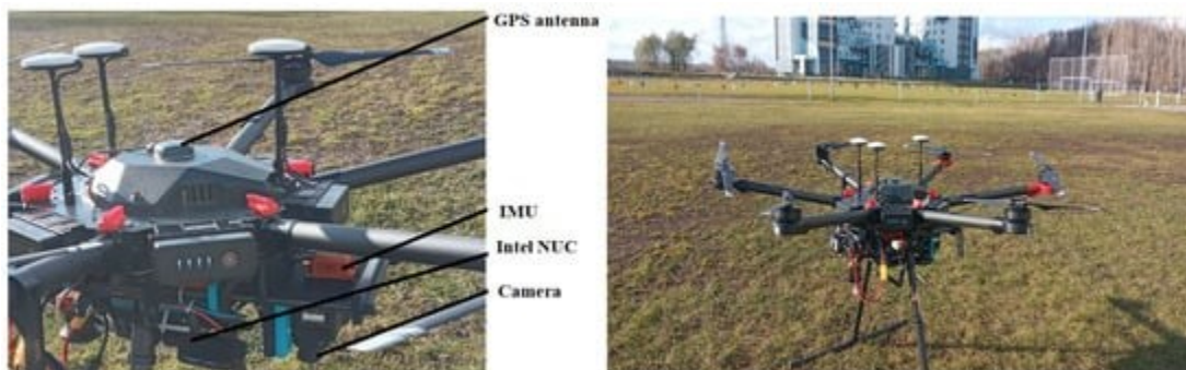
Figure 14. Example of DJI M600 integrated with customized payloads (image source: [63])
