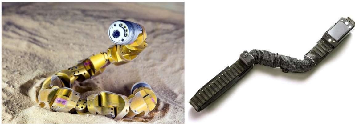
Figure 17. Examples of robots with snake-like maneuverability (left image: [64] right image: [65])
