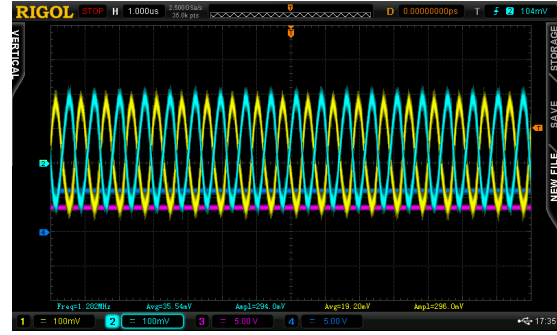
(b) 3.5V applied .015A .073W 66V RF P-P
