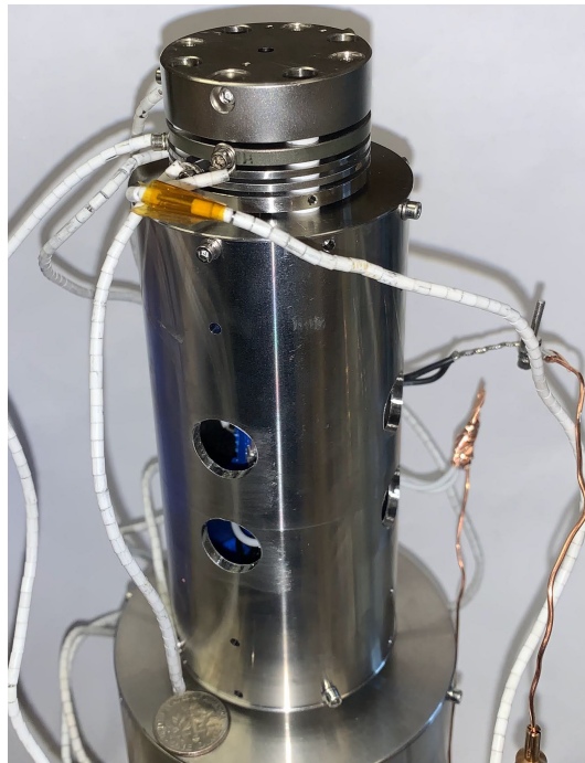
Figure 4-10: 10 cm quadrupole in metal housing with ionizer on the top and Faraday plate below. US dime coin for reference.
