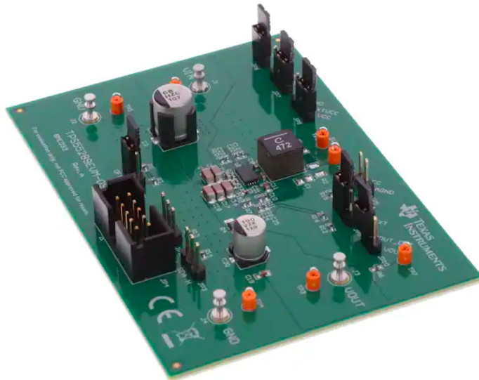
Figure 5-14: TPS55289 Buck-Boost Converter Evaluation Board to produce voltages from .8 V to 22 V [5.3]
