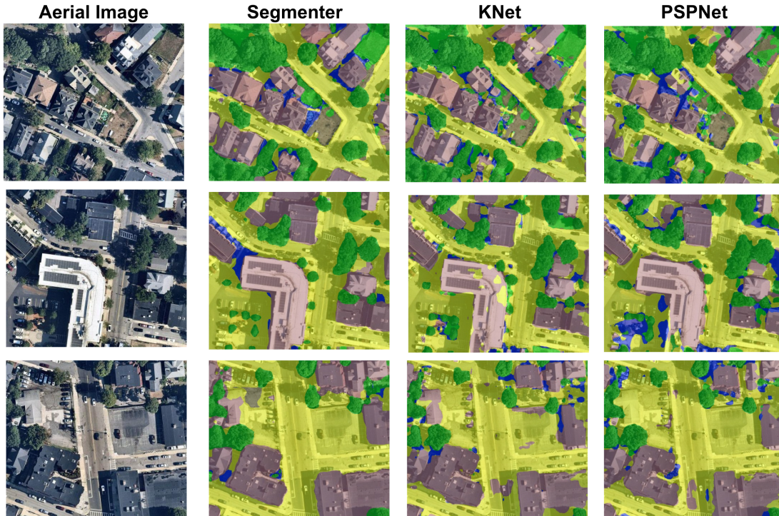
Figure 4-3: Example Segmentations of Boston Aerial Images Produced by Each Fine-tuned Model
