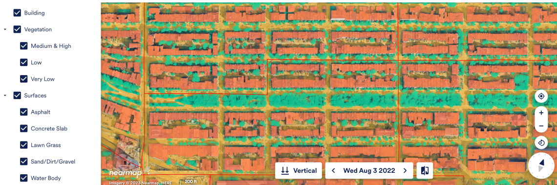
Figure 3-5: Nearmap AI Layer Features as seen on the Nearmap Map Browser. The layers on the left pane are shown in the image, where the color of the building layer is orange, vegetation layer is green, and the surfaces layer is yellow
