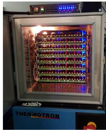
(c) Module Burn-In Test Rack
