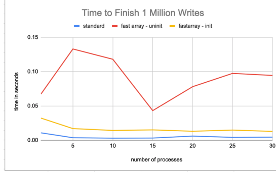
Figure 8.8.3: This plot compares the time to write to one million indices of a standard array versus a fast array for various numbers of concurrent processes. For the fast array, both writes to uninitialized and initialized indices are compared.
