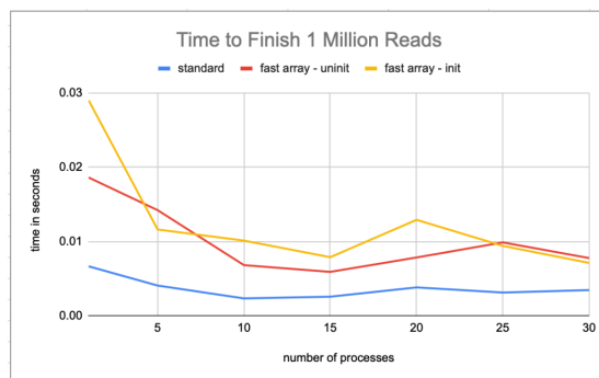
Figure 8.8.2: This plot compares the time to read from one million indices of a standard array versus a fast array for various numbers of concurrent processes. For the fast array, both reads from uninitialized and initialized indices are compared.
