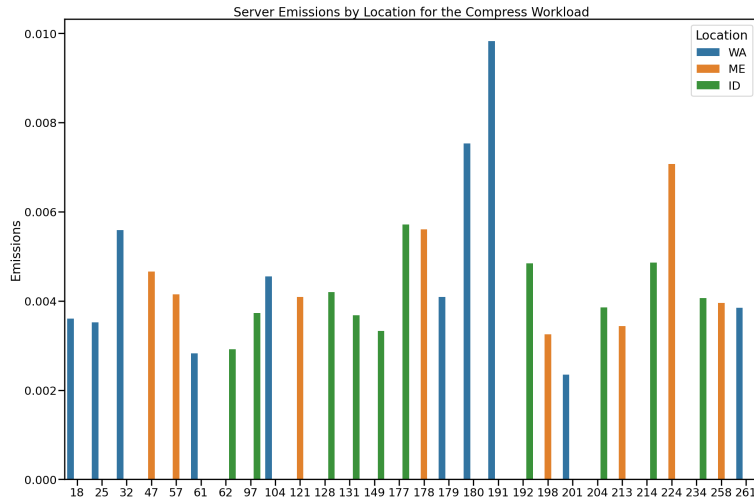
Figure 4-14: Results for scenario 3 showing the algorithm differentiating between server and data center location for the same workload. In this scenario, the three servers with the lowest emissions to complete the same task had emissions within 0.0006 lbCO 2 e of each other. Average emissions in Idaho were 0.0041 lbsCO 2 e. Average emissions in Maine were 0.0045 lbsCO 2 e. Average emissions in Washington were 0.0047 lbsCO 2 e.
