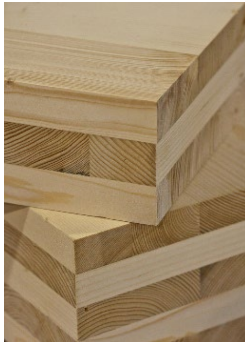
Figure 13 - Corner of CLT element (Franco, 2021)
