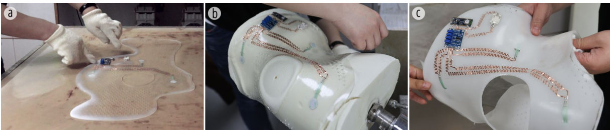
Fig. 15. Scenarios of hands-on expert study: Clinician completed the fabrication steps of heating and shaping orthosis, correcting electrode placement, and turning on the electronic function with battery installment.
