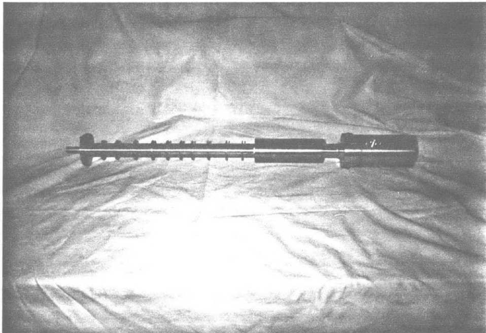
Fig. (4.13) Photograph of assembled cylinder and outer shell without surge volume.
