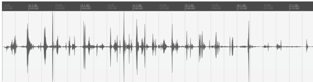
Figure 1: An audio example of eating a single Pringles chip. The recording is about 13 seconds long and each vertical line represents 1/2 second. The average RMS power is -40.2 dB. A rhythmic chewing pattern can be observed.
