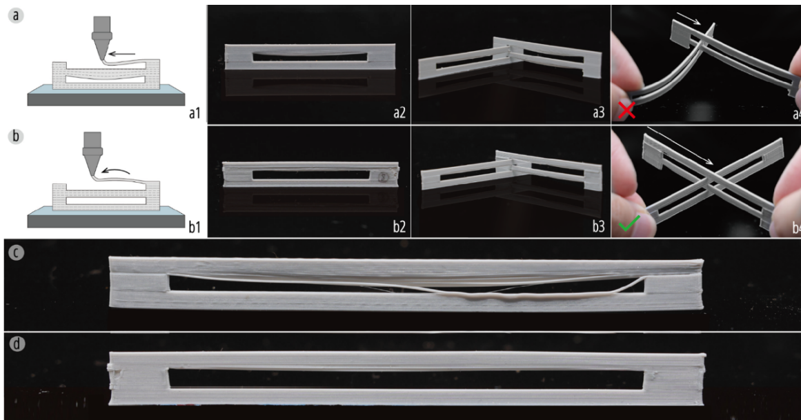
Figure 3: (a) Conventional 3D printed bridges of 50mm long and stuck result;(b) Arch-based 3D printing concept and slidably printed; (c, d) Compare two prints with a standard slicer and our method.
