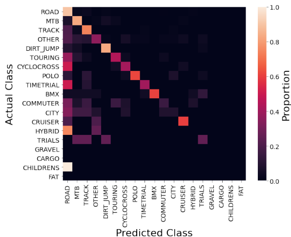
Fig. 8: Confusion matrix of parametric DNN predictions on a previously unseen test set. Actual classes are shown on the vertical axis and predictions are shown on the horizontal axis. Classes are sorted from most prevalent (top left) to least prevalent (lower right).
