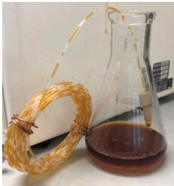
Figure 4-6: Image of gas evolution in continuous flow reactor lacking back pressure regulator.
